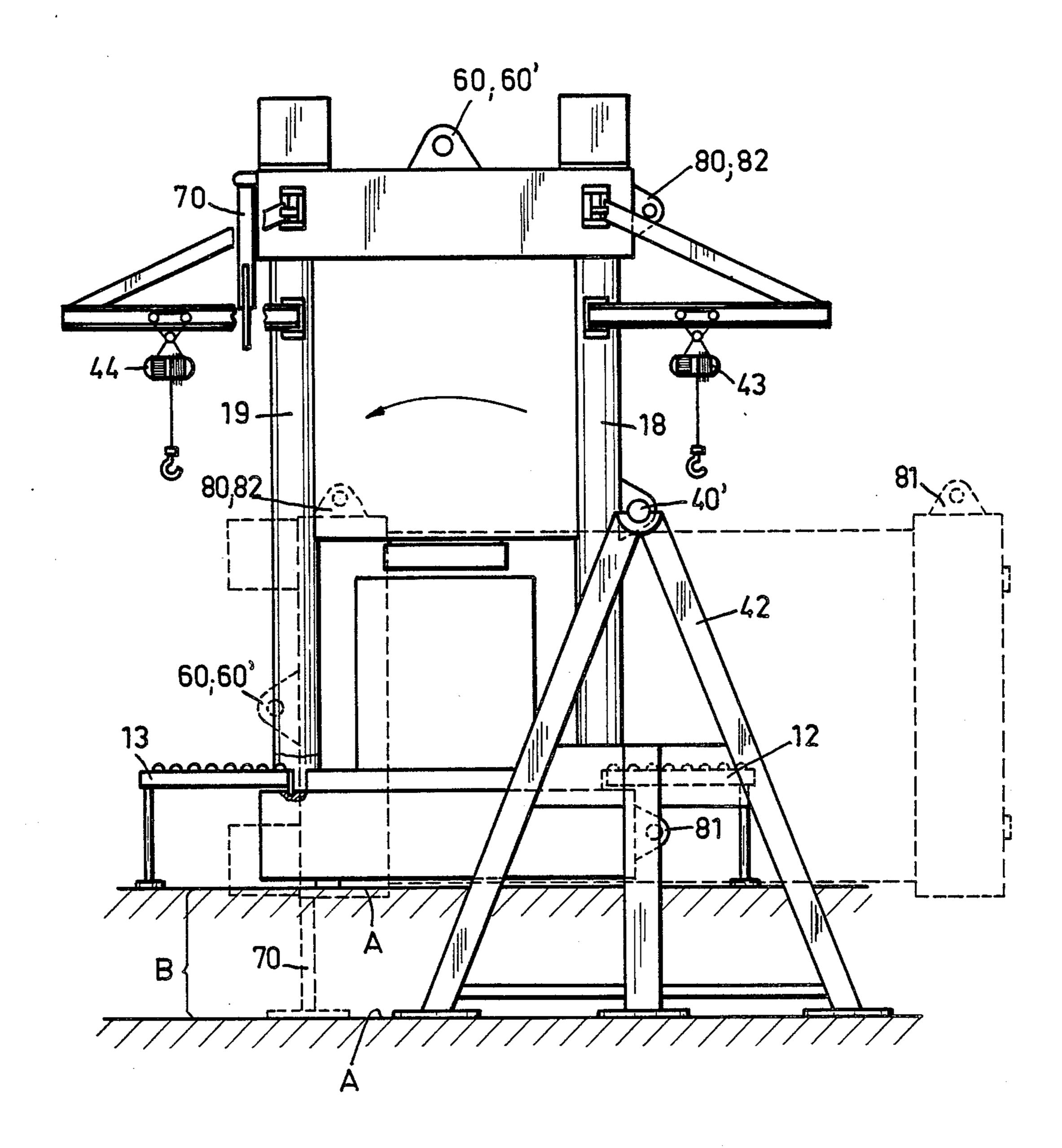
TRANSPORTABLE PRESS FOR A HIGH CONDENSABILITY OF RADIOACTIVE WASTE MATERIAL OF NUCLEAR POWER STATIONS AND PROCESS FOR CONDENSING THE SAME
