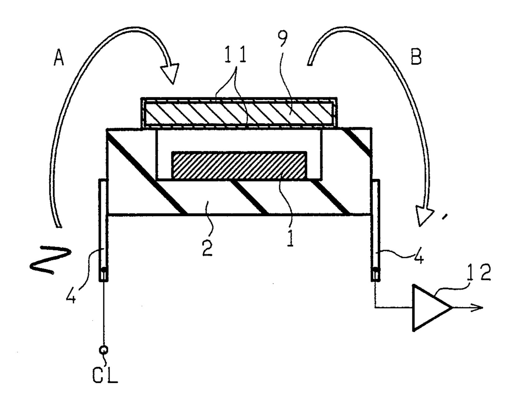
SOLID-STATE IMAGING DEVICE INCLUDING A TRANSPARENT CONDUCTOR BETWEEN AN OPTICAL LOW-PASS FILTER AND AN IMAGING **SENSOR**
