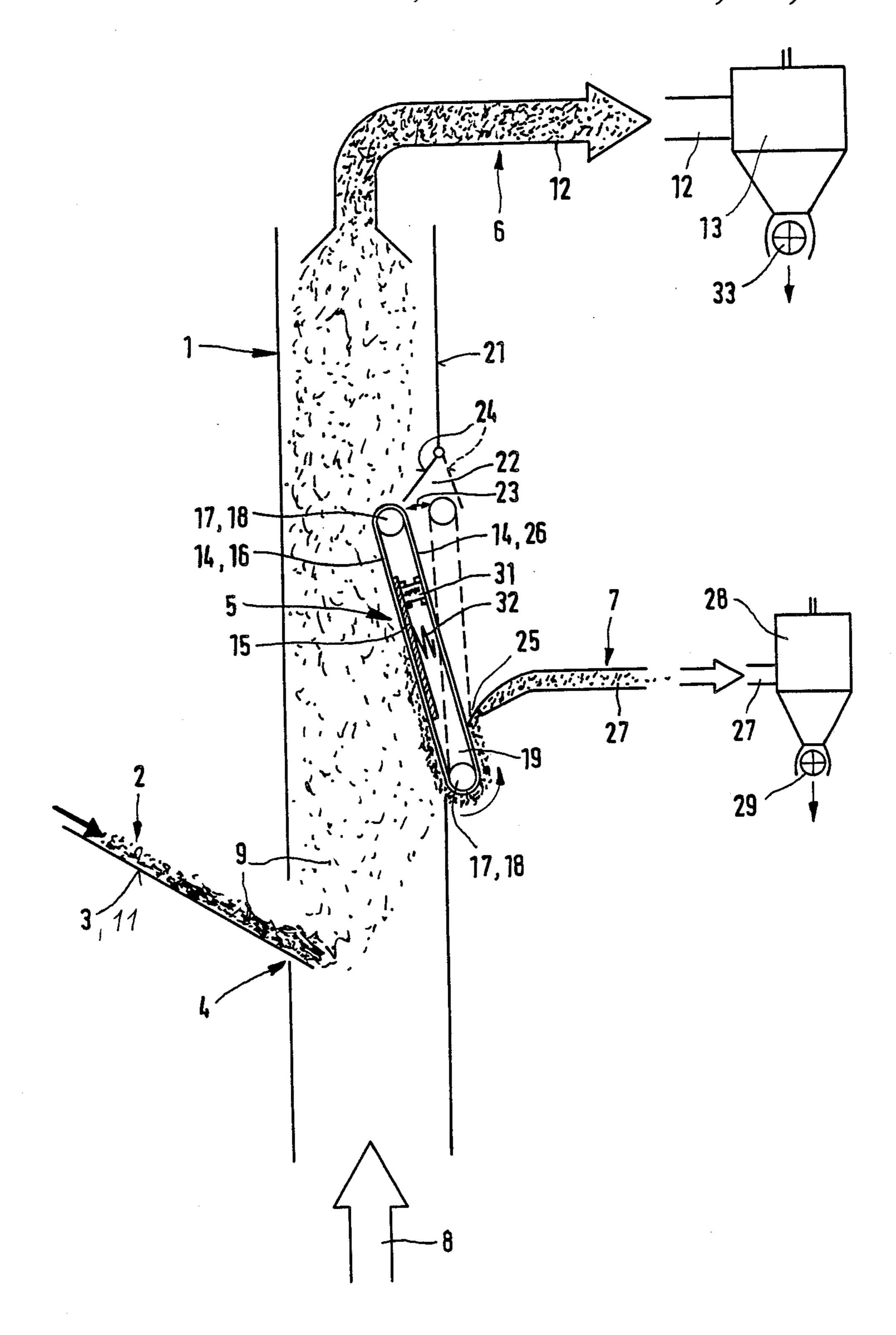
PROCESS FOR SEPARATING PARTICLES OF ELECTRICALLY NON-CONDUCTIVE MATERIAL, IN PARTICULAR PLASTICS MATERIAL AND/OR PAPER, FROM WASTE, AND A DEVICE FOR CARRYING OUT THE PROCESS
