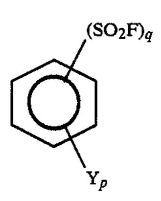
where Y is fluorine, chlorine, bromine, iodine, a methyl group, an ethyl group, or a propyl group; p is 0 to 3; and q is 2 to 6, in the presence of an alkali metal fluoride under conditions and for a time sufficient to provide a fluorinated benzene sulfonyl fluoride of the Formula (II)
