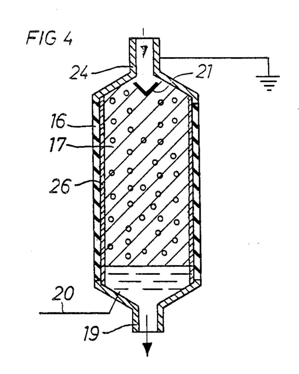
DEVICE FOR INSULATING THE SPRAY LIQUID SOURCE FROM THE HIGH TENSION VOLTAGE OF AN ELECTROSTATIC SPRAY SYSTEM WHEN USING AN ELECTRICALLY CONDUCTIVE SPRAY 5 LIQUID
