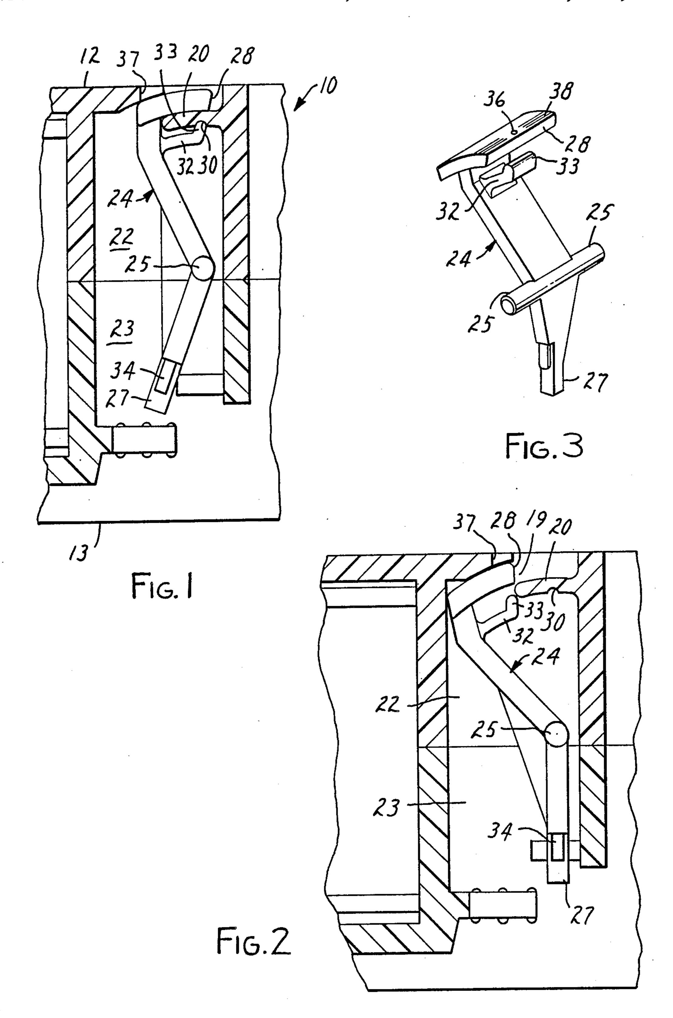
record/not record opening extending through both an under wall of the cassette and a top wall which is visible
