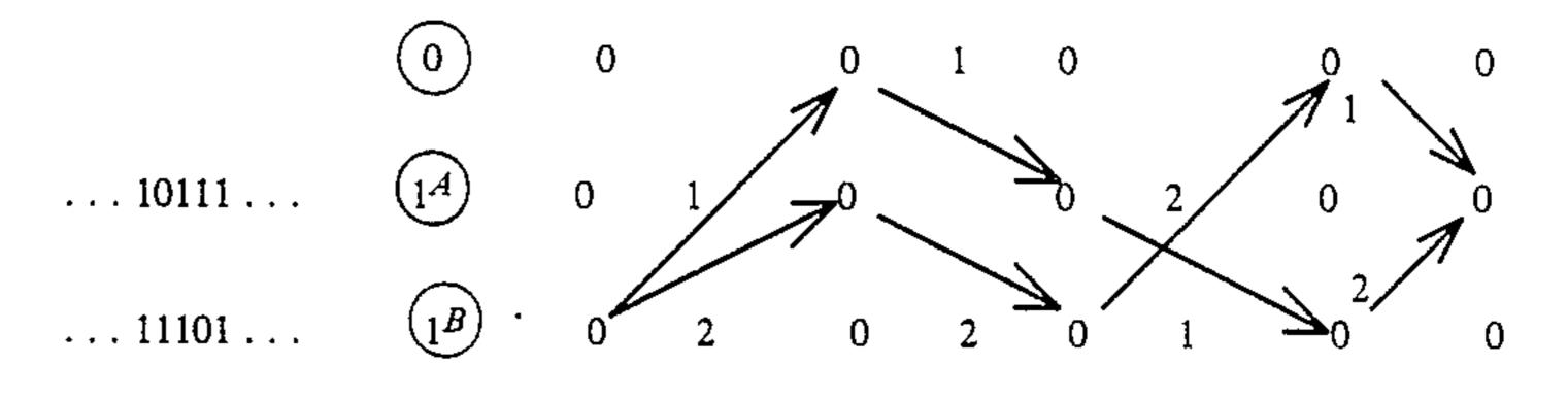
thereby producing a near maximum-likelihood estimate (or most probable EMM sequence) of the transmitted original data sequence supplied via bus 10. A decoder 40 14 then generates, from the detected sequence, the EMM code output data in a bus 15. The decoder 14 is a sliding block decoder with a window size of ten code bits, providing maximum error propagation of no more than eight user bits.
