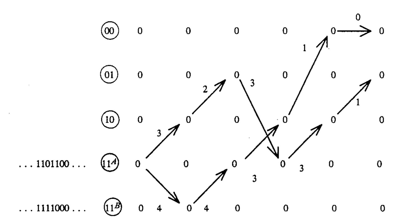
The increase in free distance for the  $(1+D)^2$  channel 20 thus represents a coding gain, unnormalized for rate loss, of
