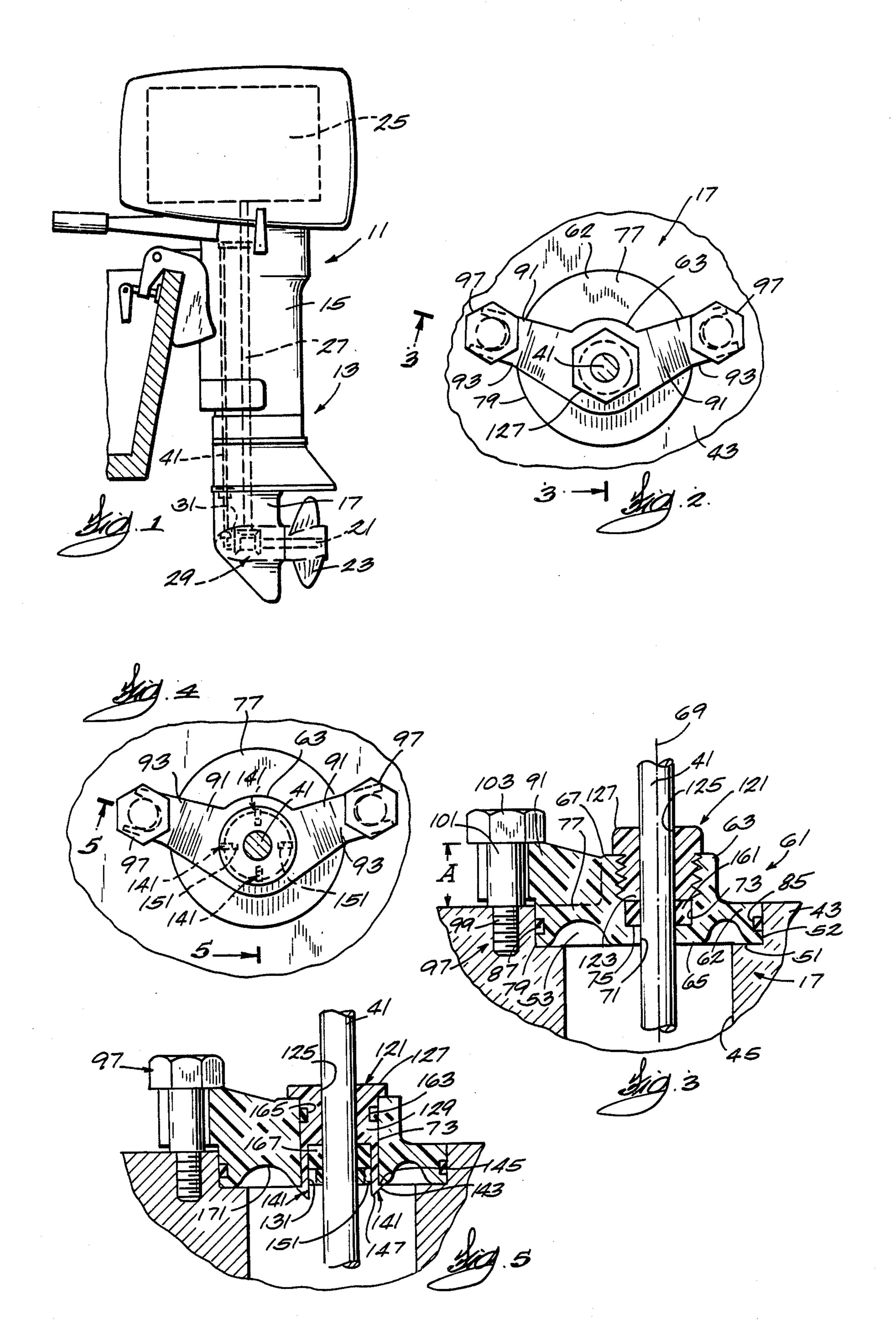
COMBINED SHIFT ROD BUSHING AND GEAR CASE SEAL FOR MARINE PROPULSION DEVICE
