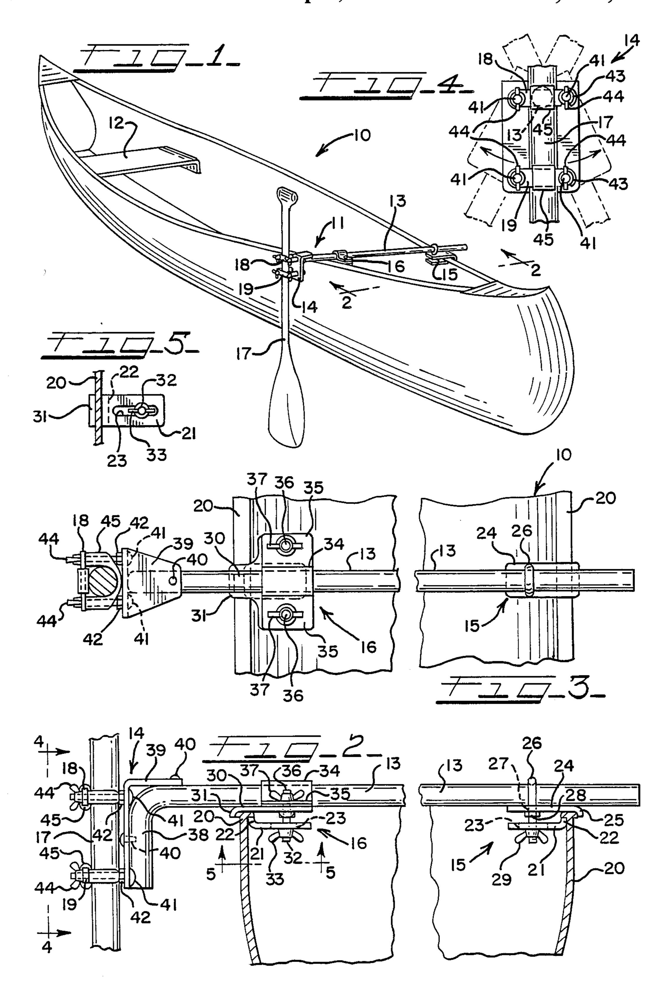
CANOE STABILIZING AND GUIDE MECHANISM
