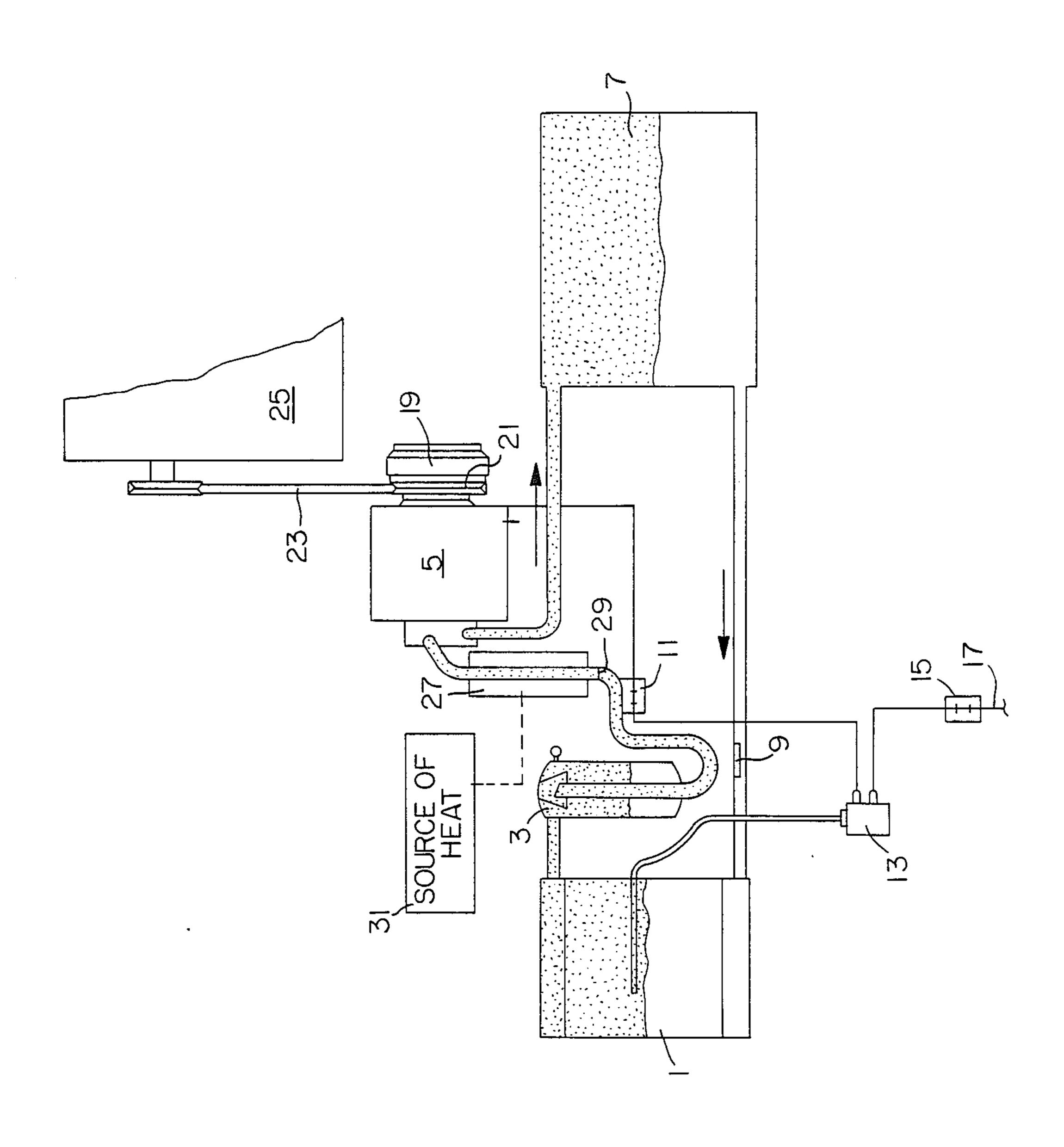
the compressor, heating commences and when the compressor is again engaged, heating is stopped.
