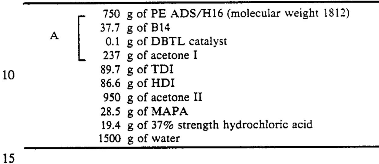
A prepolymer solution having an NCO content of 0.76% is prepared as described in Example 1. Thereafter, chain extension is carried out, the salt is formed, the product is dispersed in water and finally the acetone is distilled off, these steps being carried out as described in Example 2.
