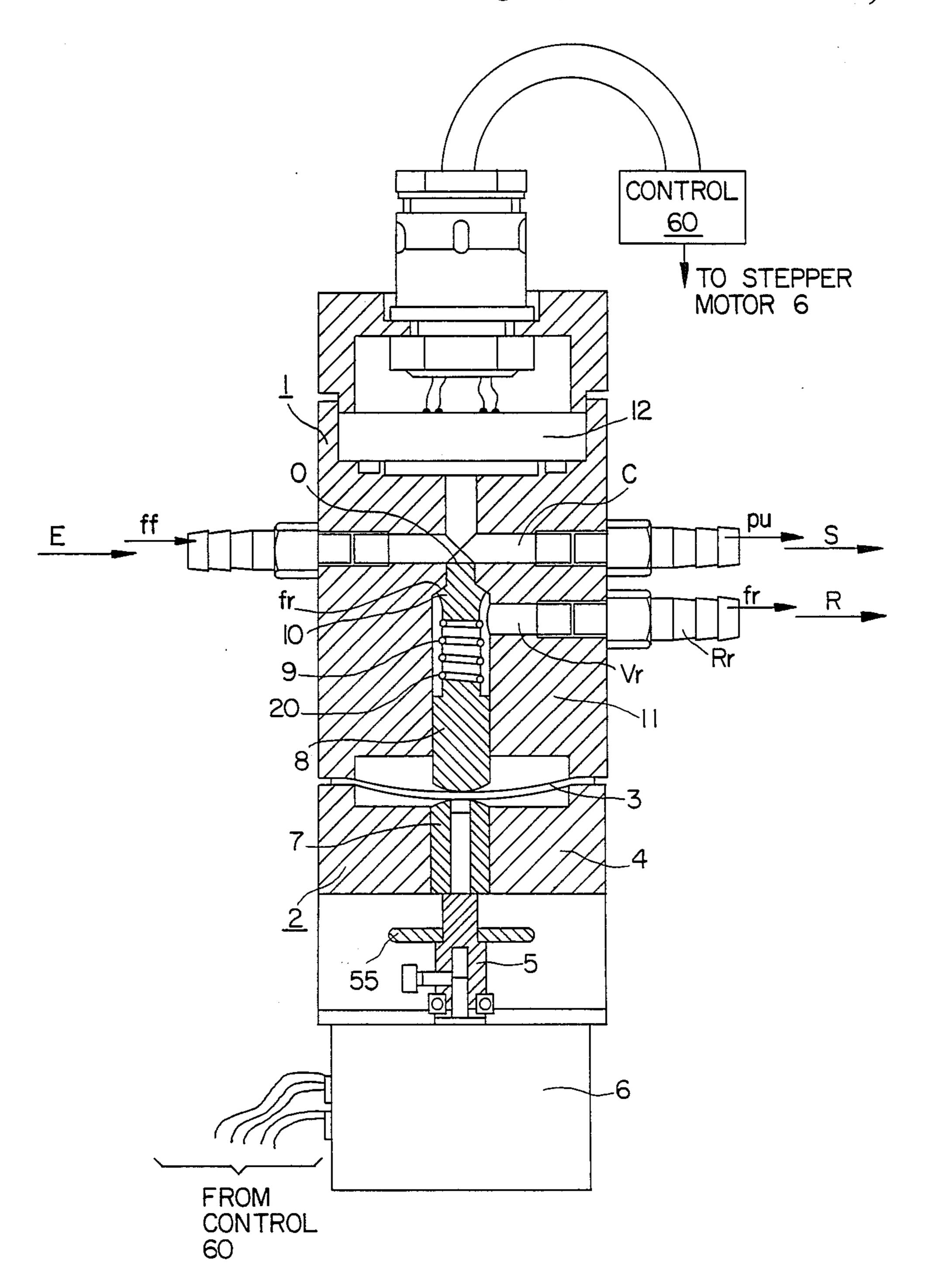
With the top of this "fluid section" 1 is associated a pressure sensing cell 12 which provides permanent reading of the user pressure obtained pu.
