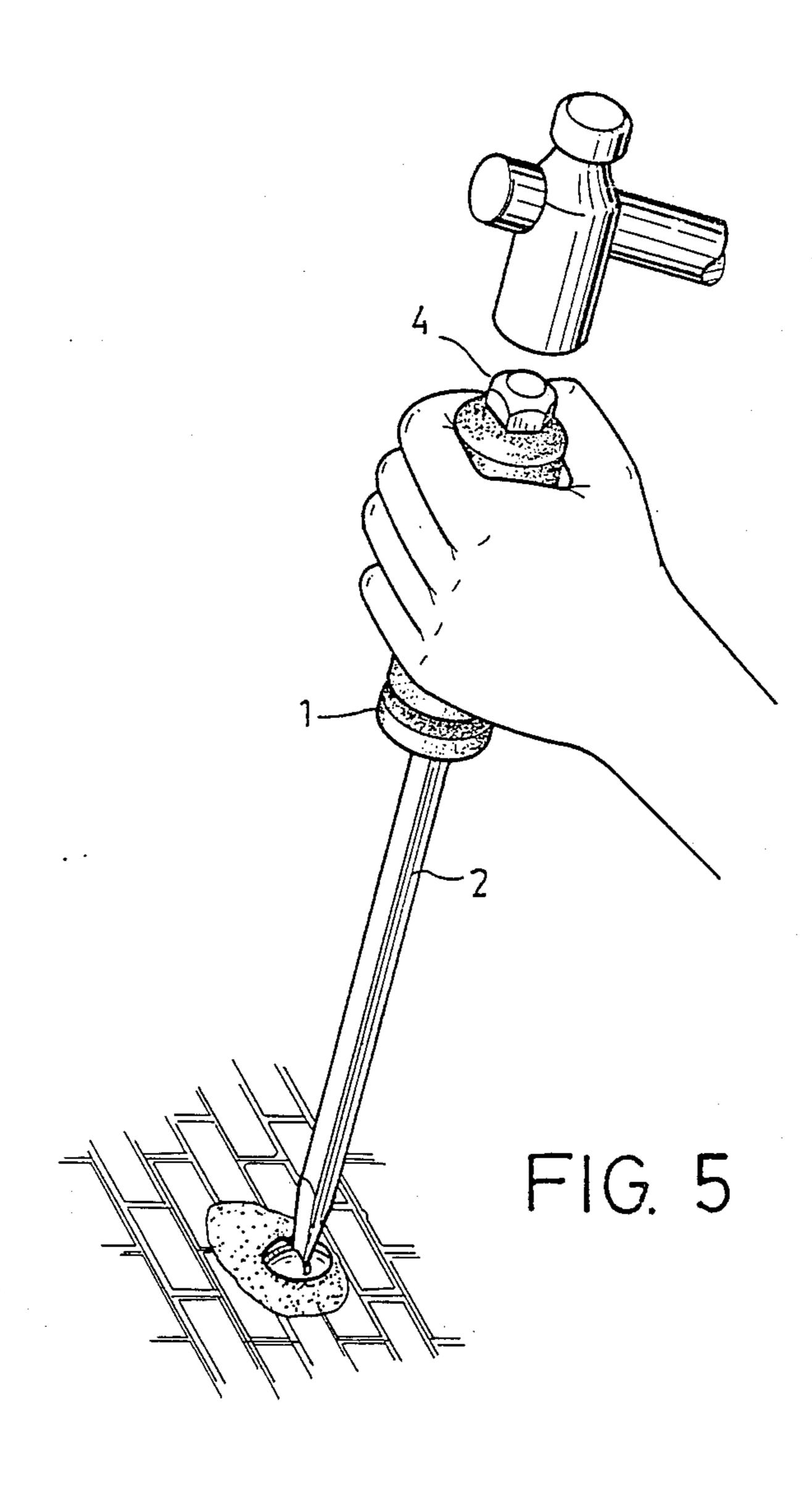
SCREWDRIVER WITH INSULATED SHAFT AND POLYGONAL DRIVING HEAD
