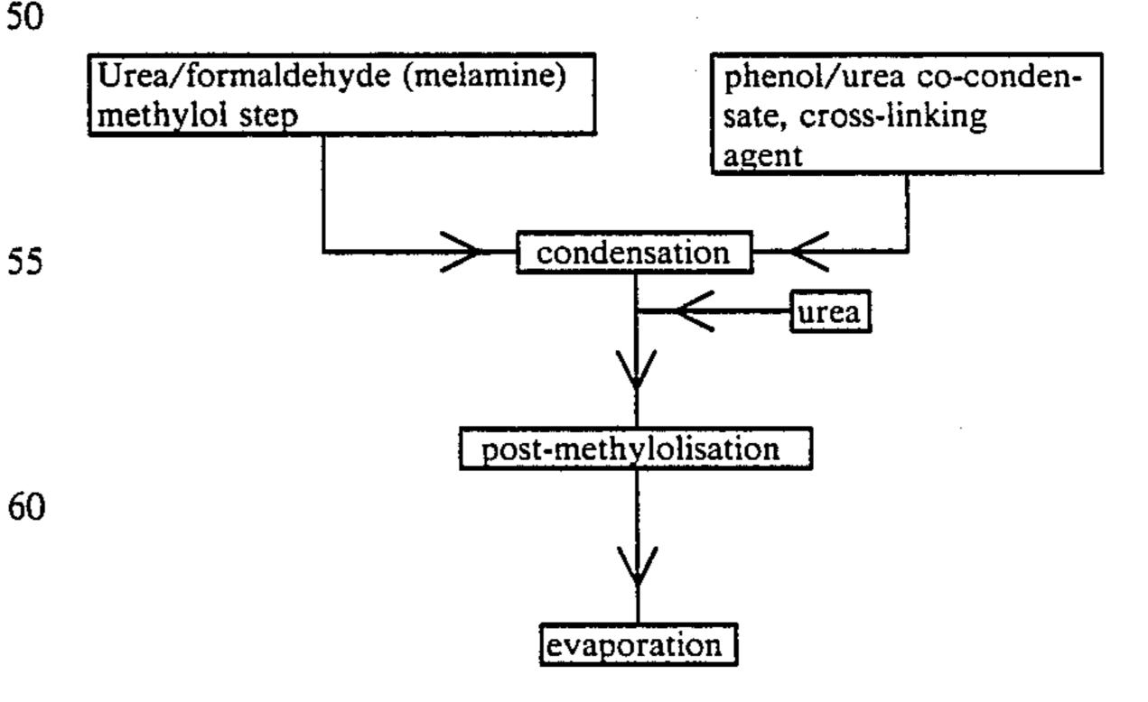
Even when the cross-linking agent is added in the form of methylol phenol and corresponding amount of urea as in the phenol/urea co-condensate above, the addition is made in the process step wherein the resin
