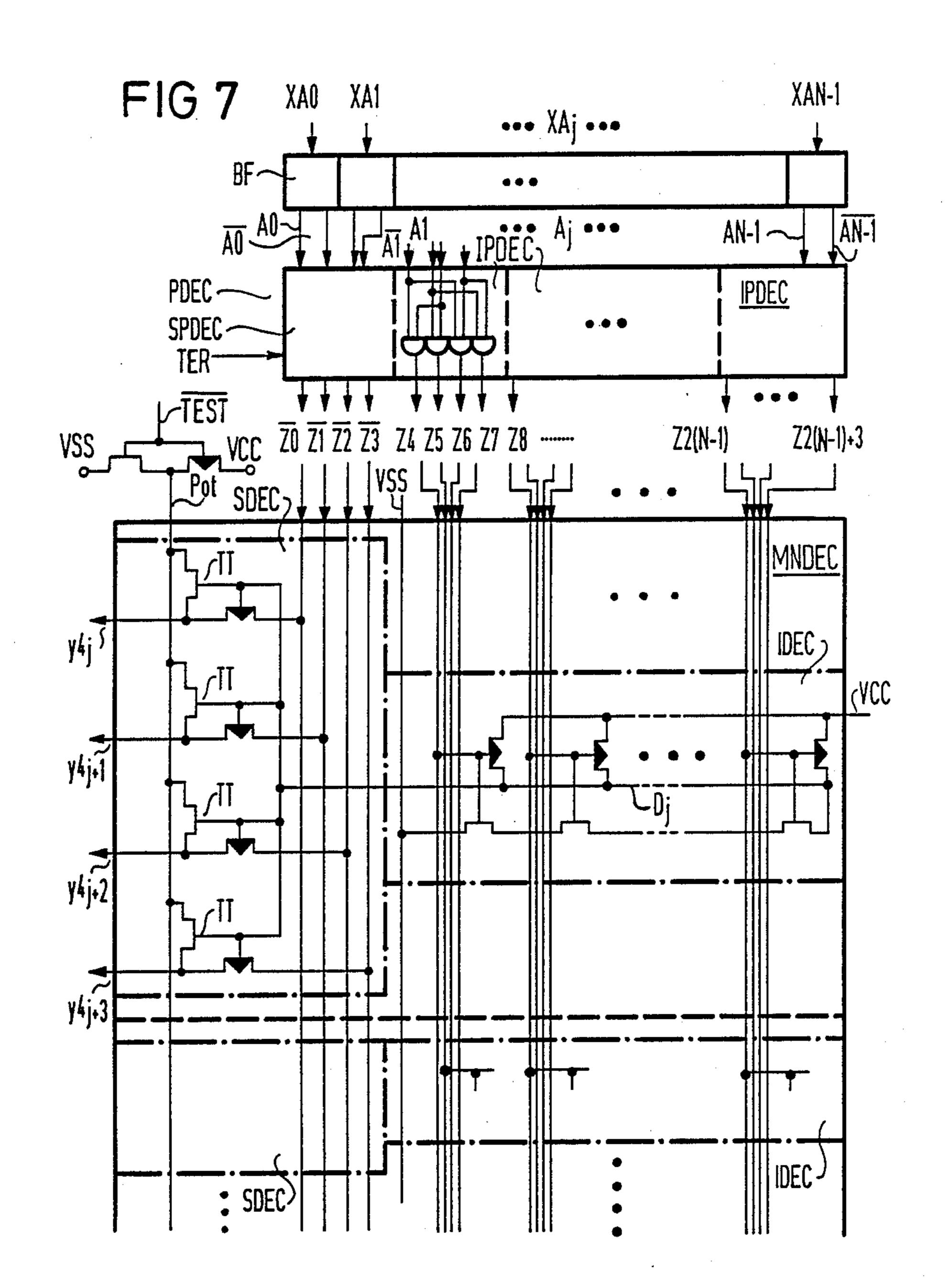
selection decoders each having connected through the source terminals of a respective one of the transfer transistors to the second potential line.
