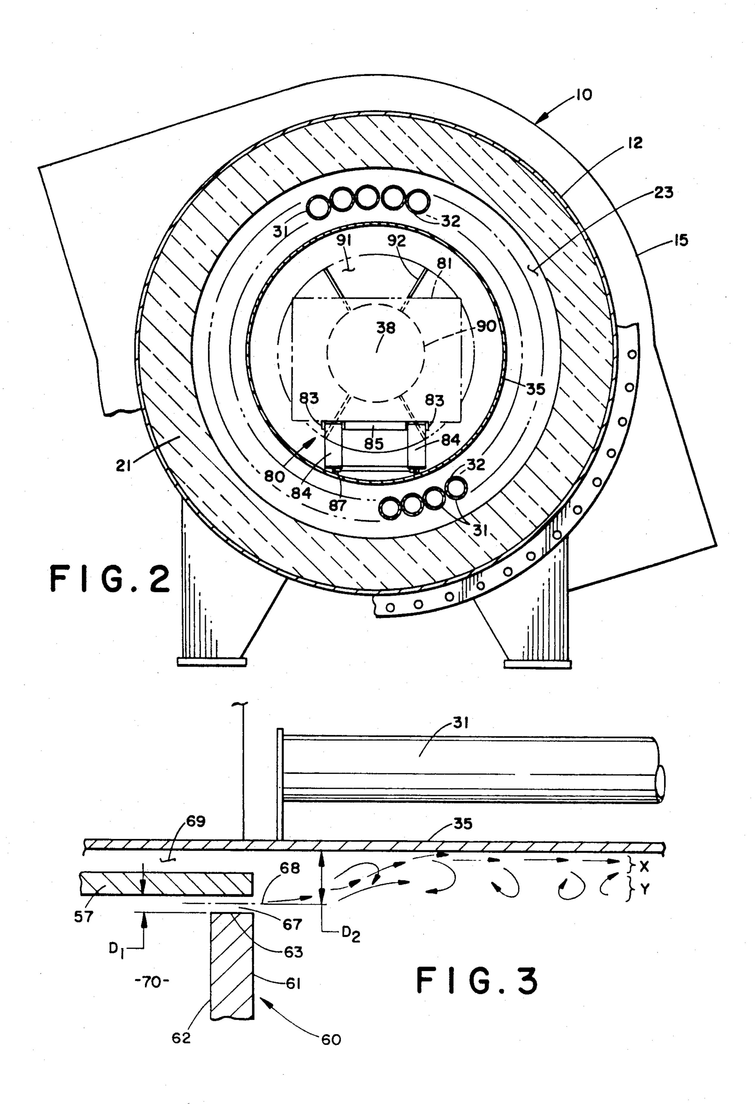
CONVECTIVE HEAT TRANSFER WITHIN AN INDUSTRIAL HEAT TREATING FURNACE
