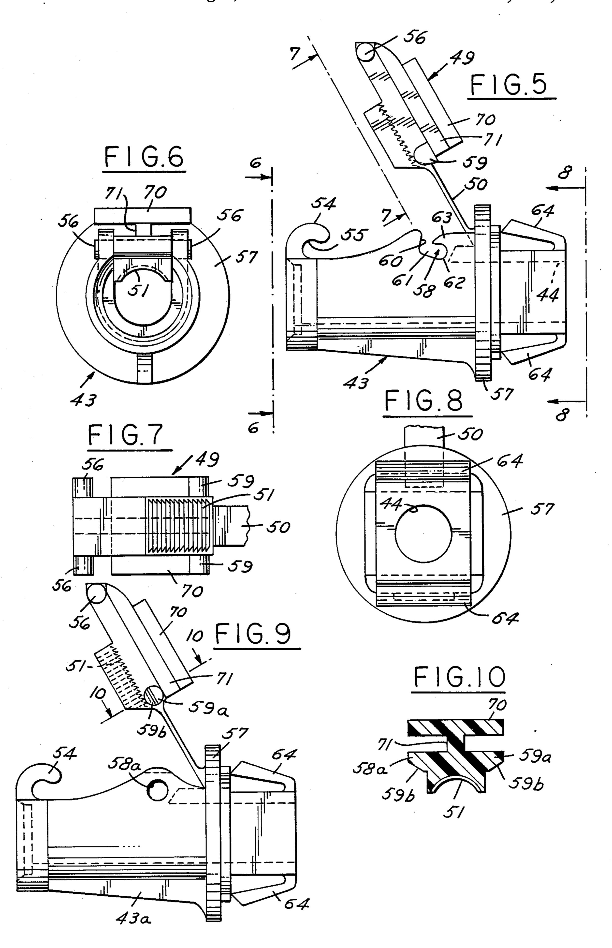
body and adapted to be moved into position to cause teeth thereon to engage the teeth on the slider. The locking member has other portions thereof which engage the body for locking the locking member in position.
