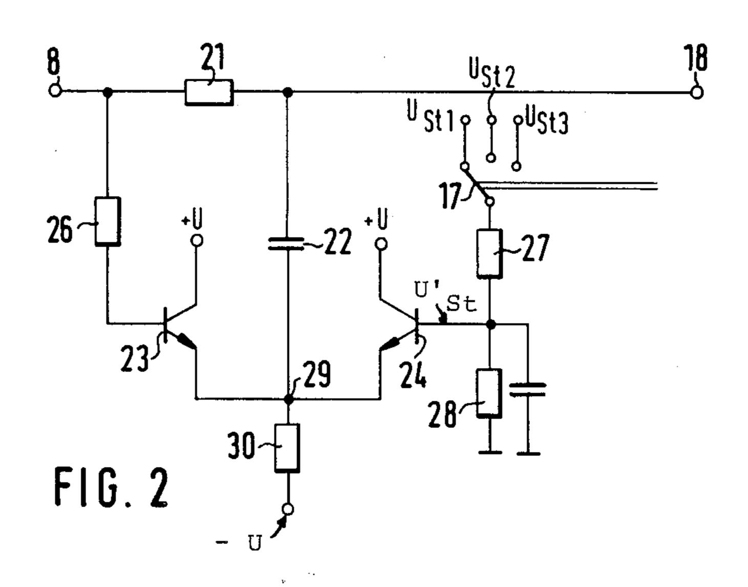
FIG. 2 is a detailed circuit diagram of the noise reduction circuit.
