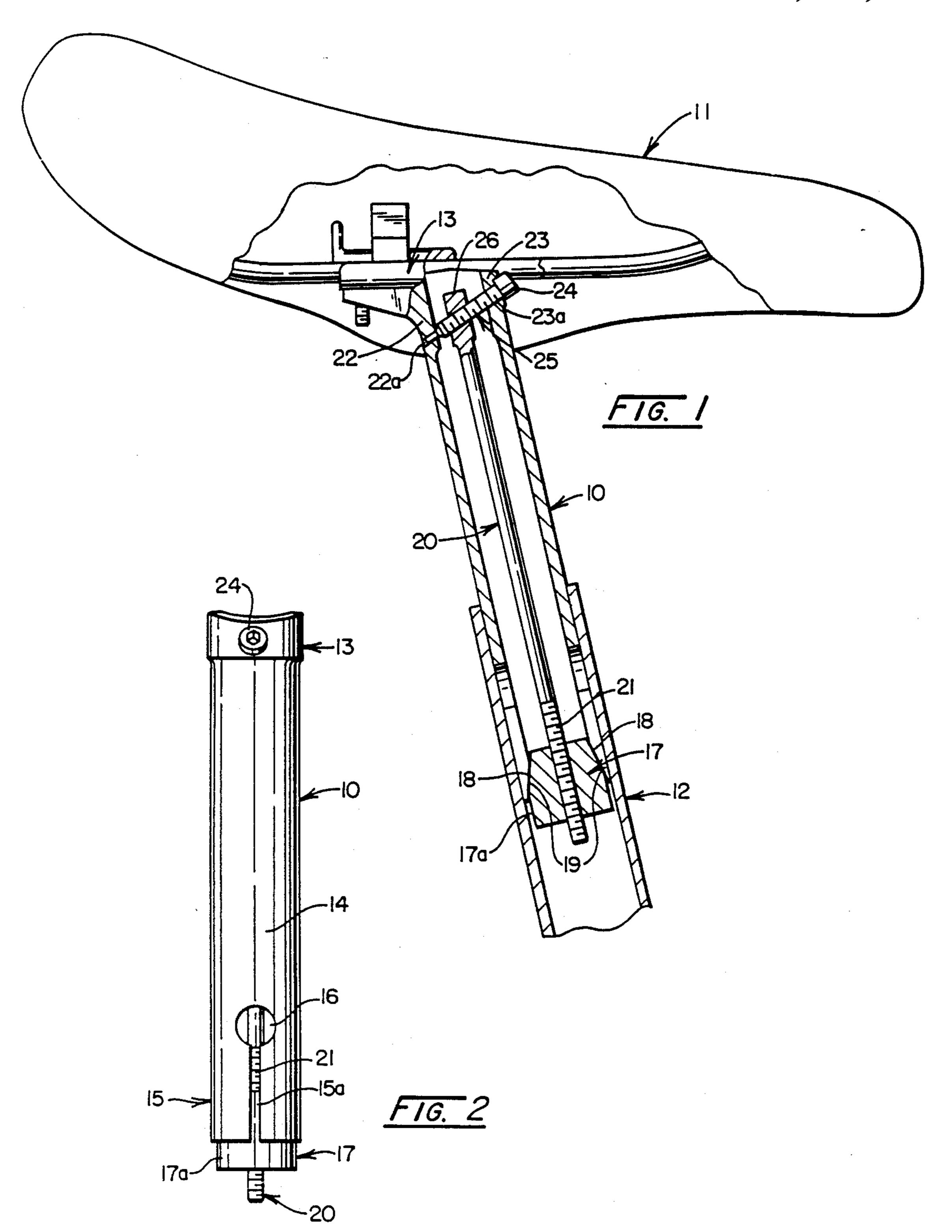
the expandable post end or collar could be made in other ways to be capable of expansion transversely into tight contact with the socket of the tube 12.
