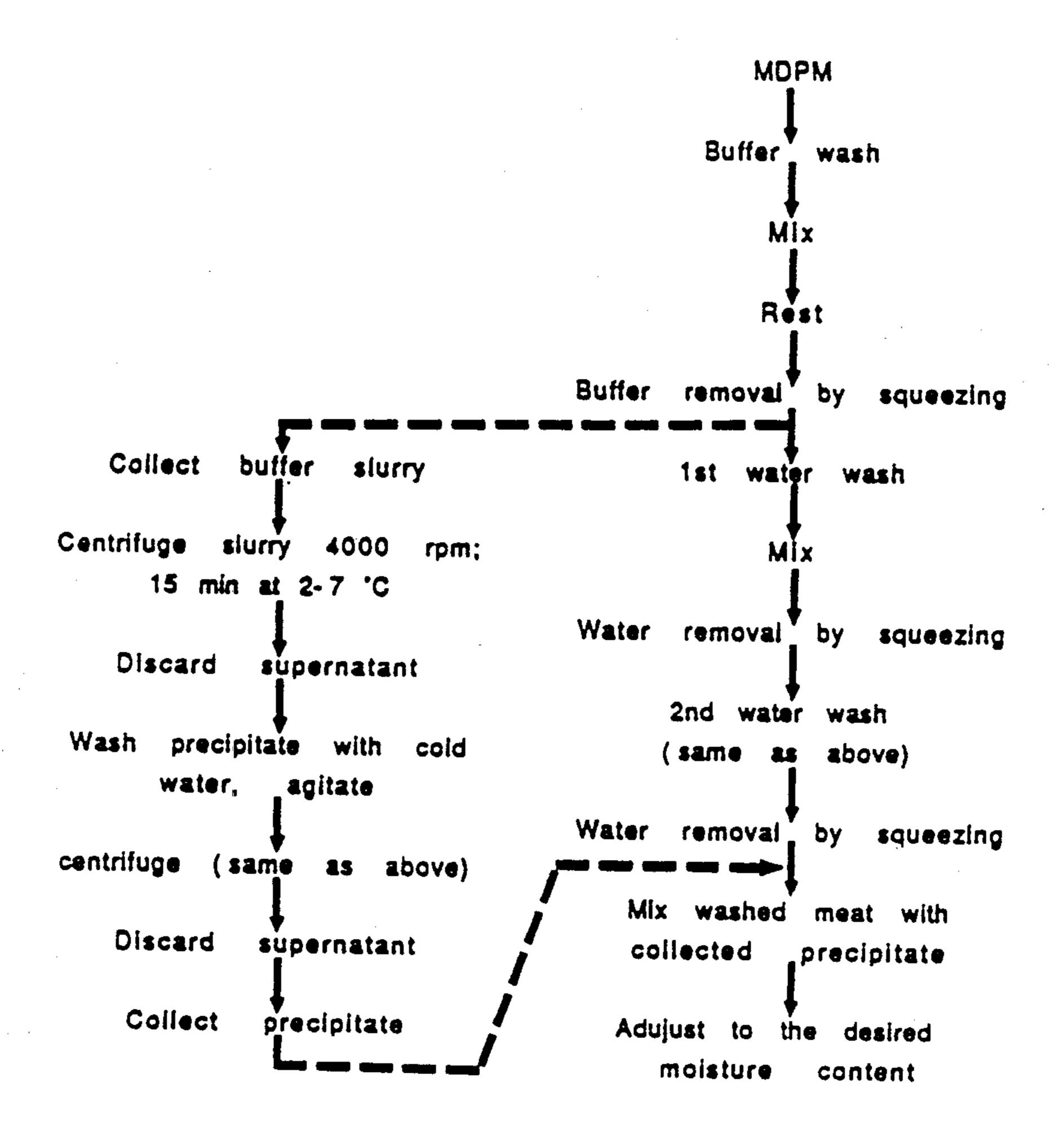
Figure 1: Flow diagram of the washing process incorporating the centrifugation of the buffer slurry
