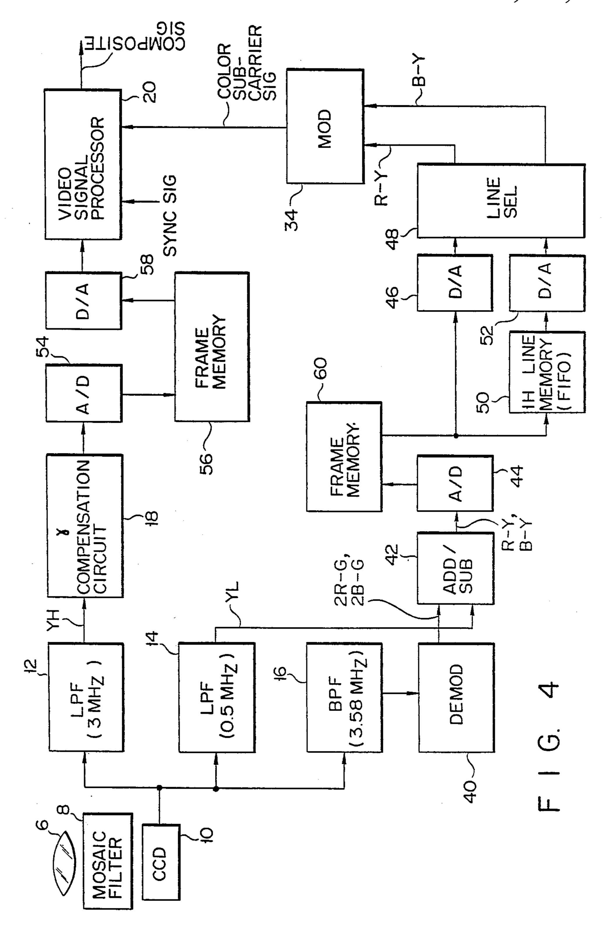
COLOR IMAGE SENSING APPARATUS WITH MEANS FOR ALTERNATELY EXTRACTING FIRST AND SECOND COLOR DIFFERENCE SIGNALS INCLUDING A FIRST-IN FIRST-OUT DIGITAL LINE MEMORY
