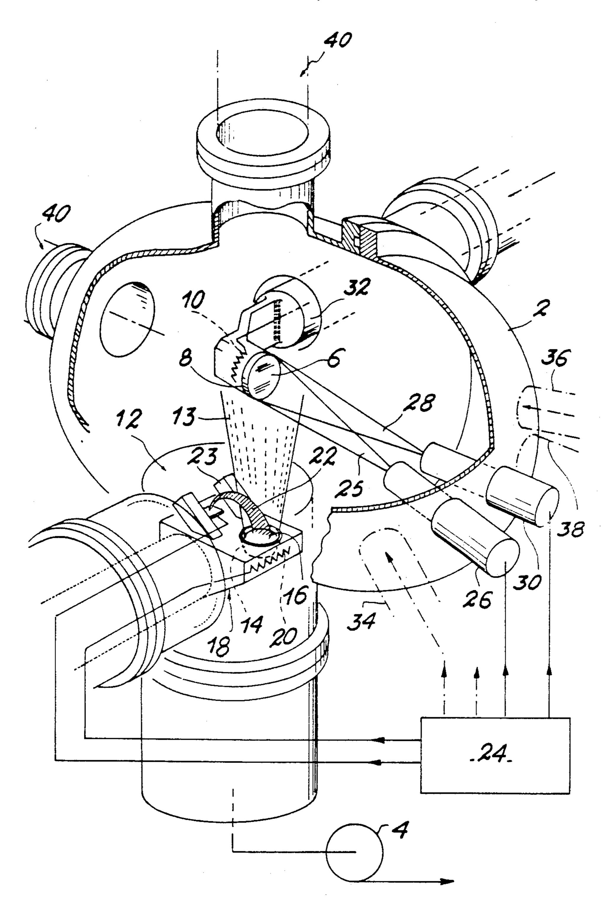
PROCESS FOR THE DEPOSITION BY EPITAXY OF A DOPED MATERIAL
