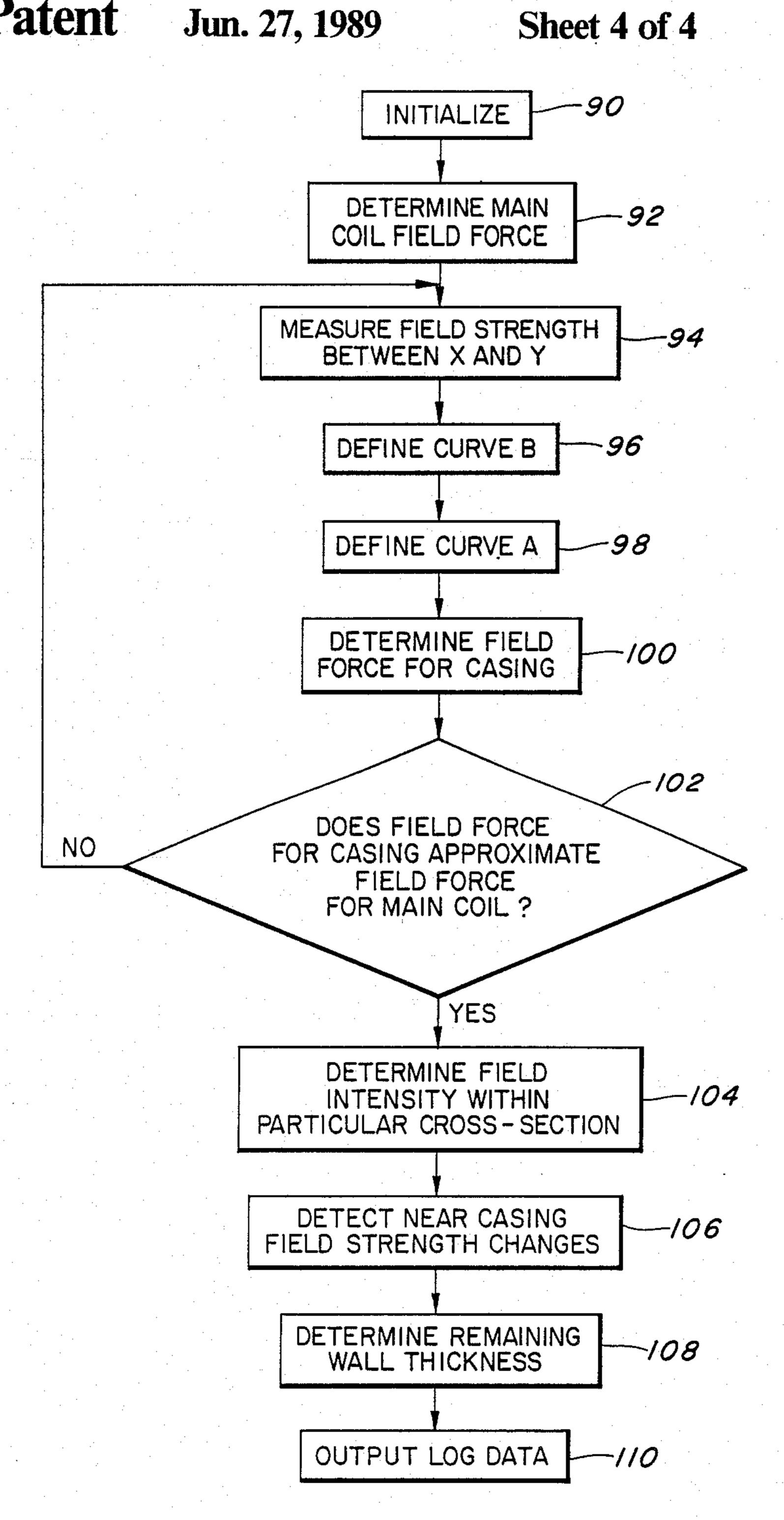
METHOD AND APPARATUS FOR MEASURING CASING WALL THICKNESS USING A FLUX GENERATING COIL WITH RADIAL SENSING COILS AND FLUX LEAKAGE SENSING COILS
