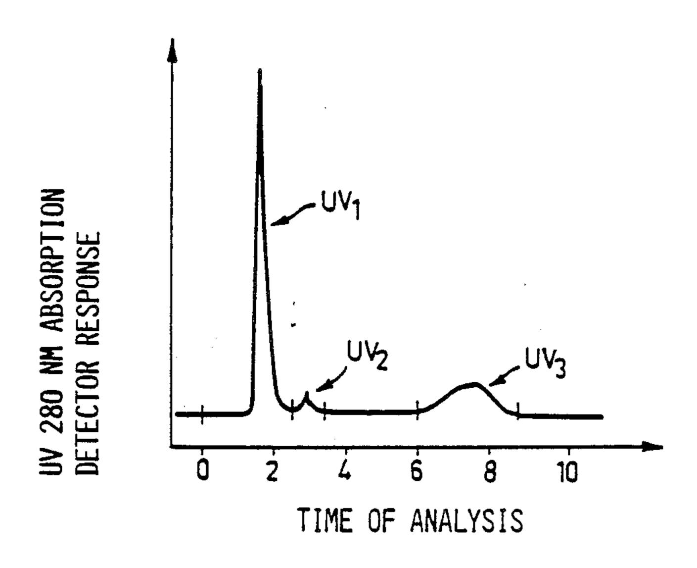
ANALYSIS OF A SULPHITE COOKING LIQUOR SAMPLE FOR THE LIGNIN, TOTAL SULPHUR DIOXIDE AND FURFURAL THEREOF BY MEANS OF AN AUTOMATIC ANALYZER
