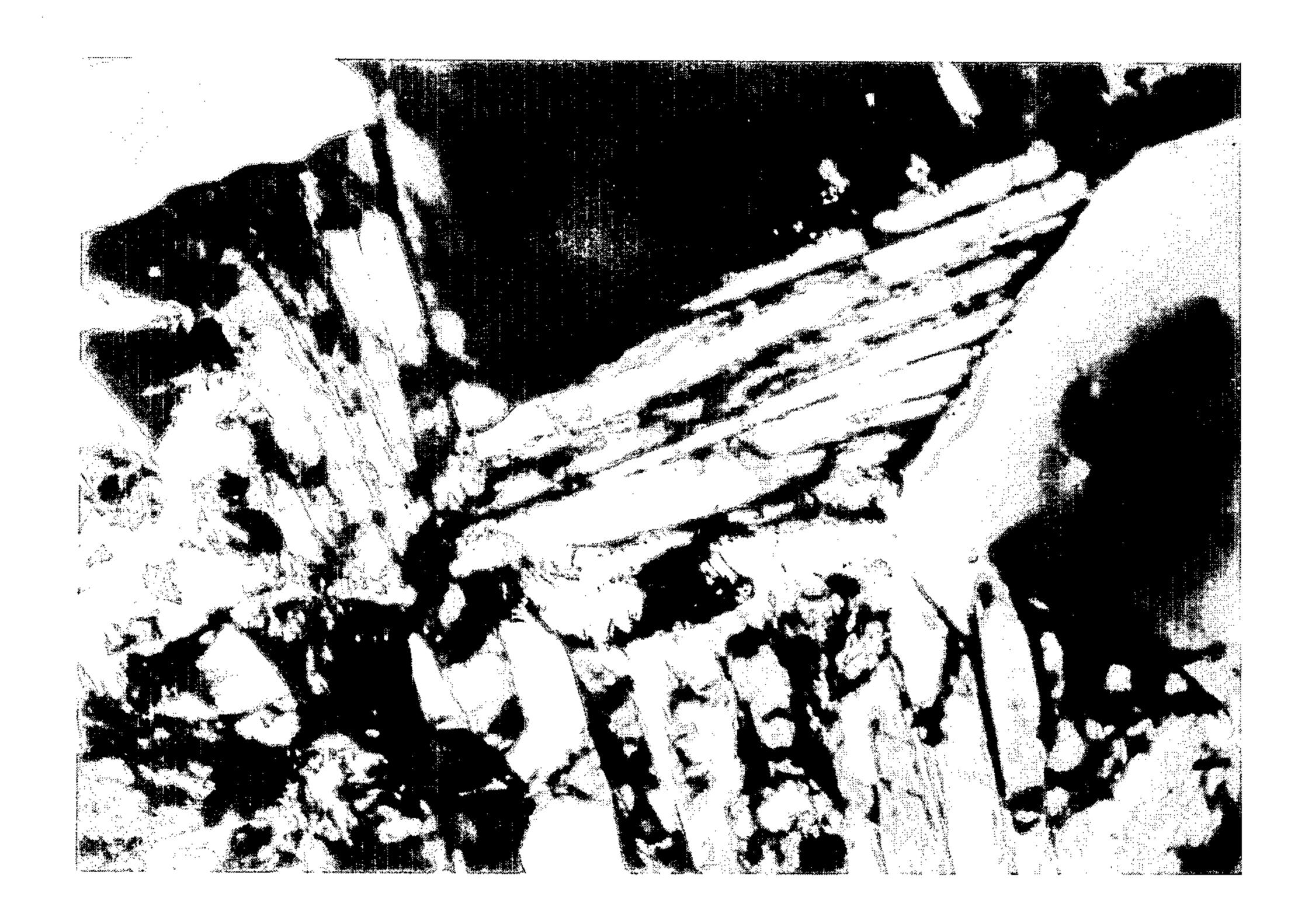
TEM picture fine  $(\alpha + \beta)$  structure 975 °C/3 min/water + 500 °C/2 h 64 % deformed at 850 °C
