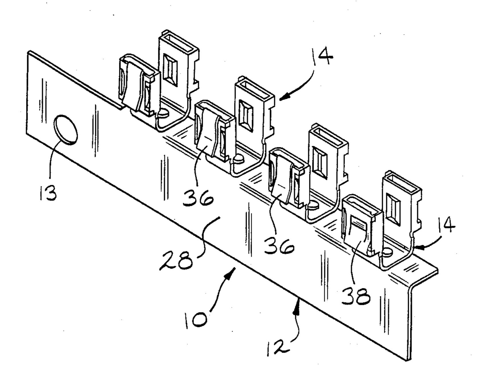
bus bar assembly may be mounted within a plastic connector housing which then is bolted to the vehicle.
