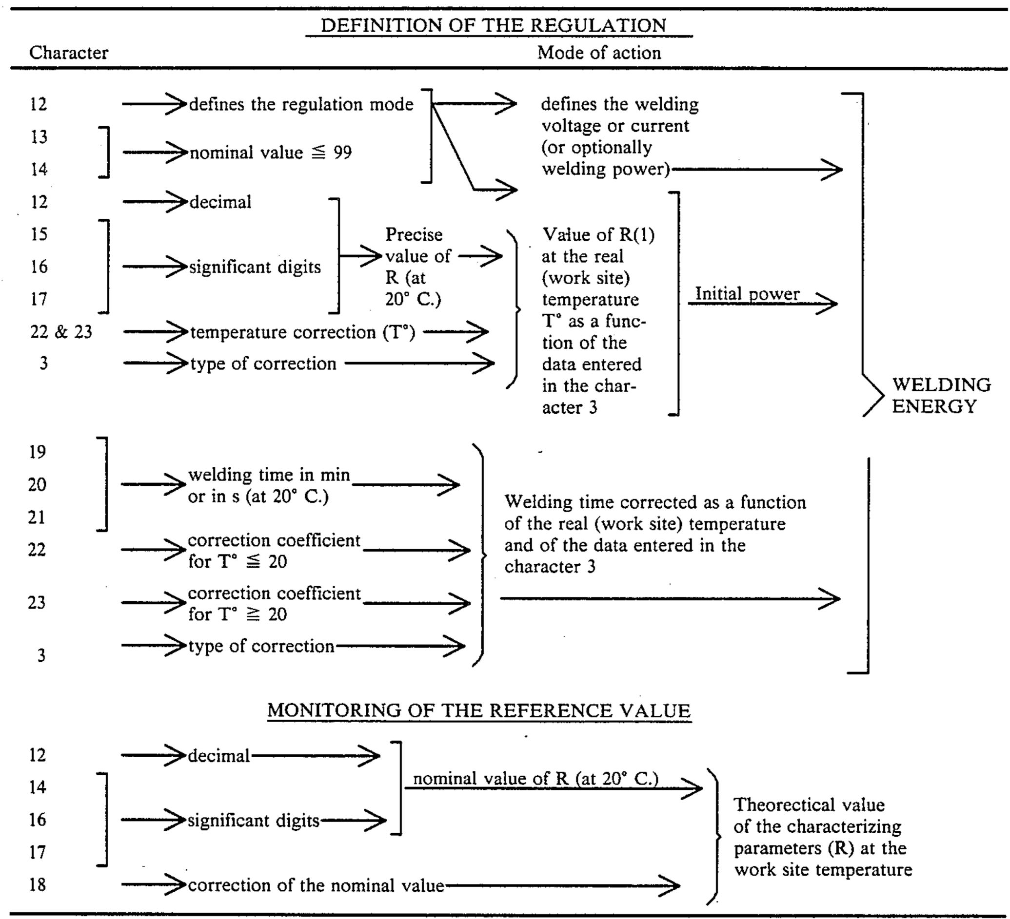
Note: the nominal reference temperature (T°) has been arbitrarily taken as being 20° C. (1) R = characterizing parameter "resistance of the component" considered
