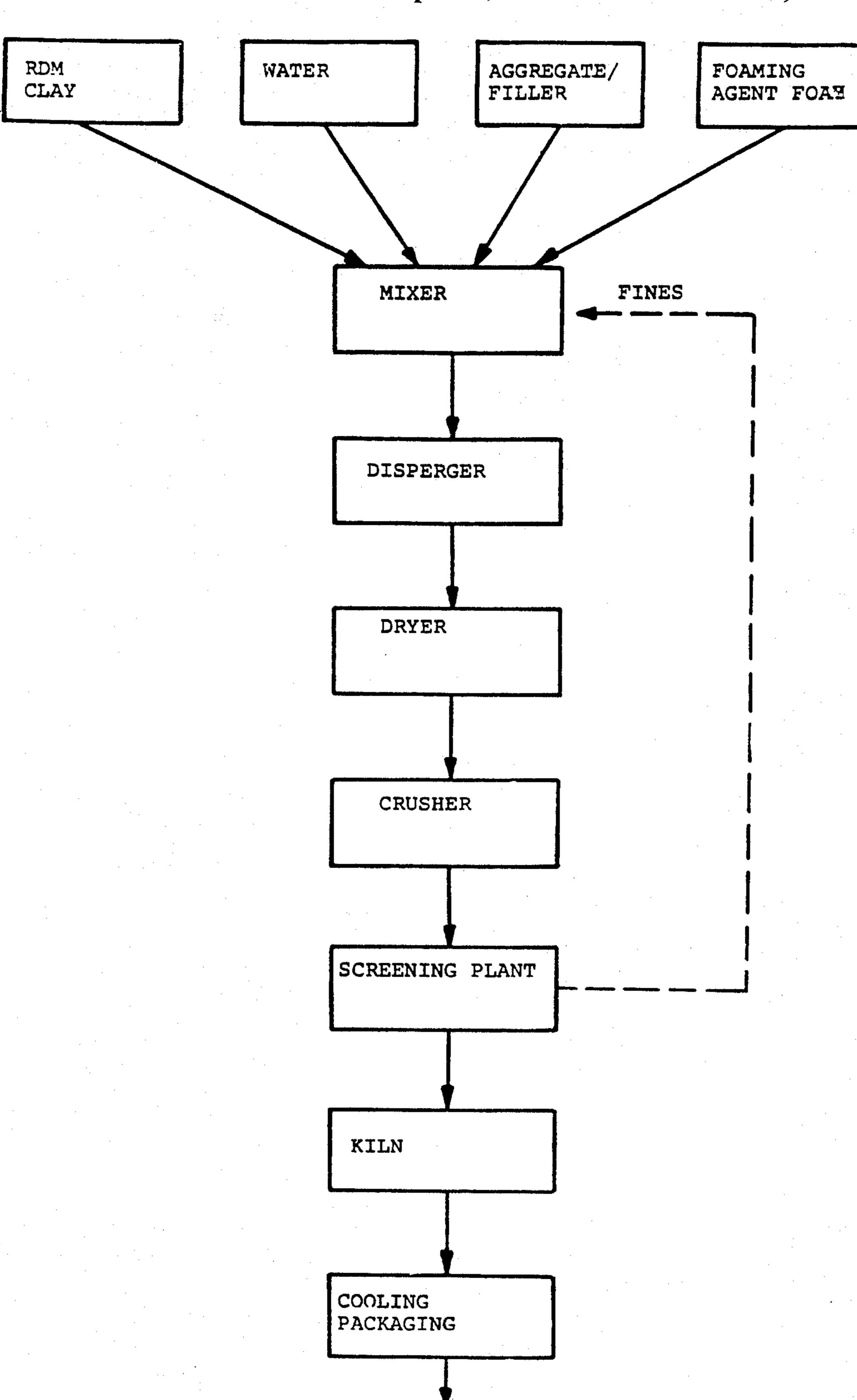
HIGHLY POROUS CERAMIC MATERIAL FOR ABSORPTION AND ADSORPTION PURPOSES, PARTICULARLY FOR ANIMAL LITTER/BEDDING, PROCESS FOR THE PRODUCTION THEREOF AND THE USE THEREOF
