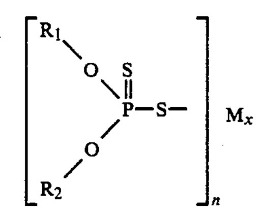
wherein n is 1-6; x is 1-3; R<sub>1</sub> and R<sub>2</sub> may each be hydrogen or a hydrocarbyl group having from 1 to 30 carbon atoms; and M is a metal selected from the group consisting of aluminum, antimony, cadmium, copper, lead, tin, 20 zinc and mixtures thereof, in which the metal is different in at least two compounds.
