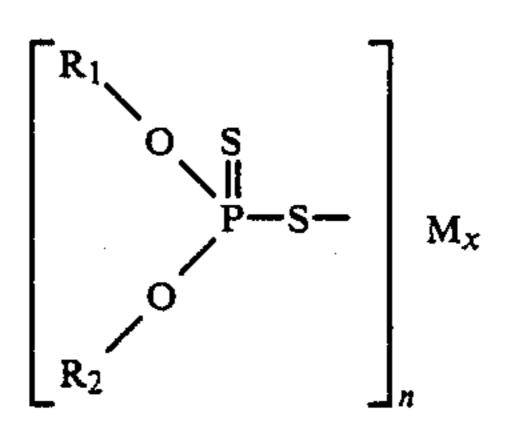
wherein n is 1-6; x is 1-3;  $R_1$  and  $R_2$  may each be hydrogen or a hydrocarbyl group having from 1 to 30 carbon atoms; and M is a metal selected from the group consisting of aluminum, antimony, cadmium, copper, lead, tin, zinc and mixtures thereof.
