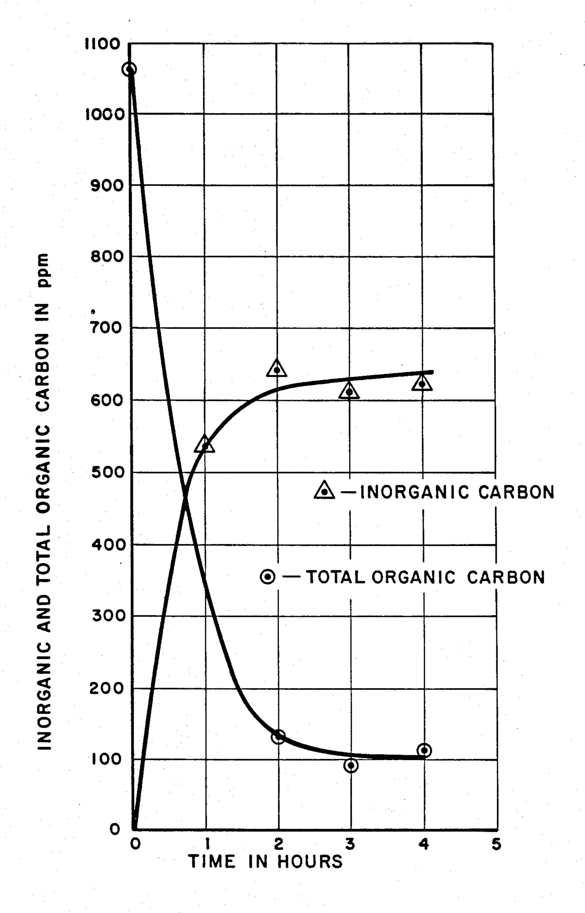
Fig. 7 PERCENT M71 OXIDIZED USING 4M H<sub>2</sub>O<sub>2</sub> AT pH 12.5
