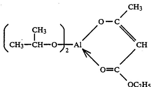
According to the present invention, the coupling agent is preferably contained in the amount of 0.3% by volume based on the total volume of the composition. When the amount of the coupling agent is less than 0.3% by volume, the polymer cannot completely surround the magnetic powder particles, resulting in poor insulation and an unsatisfactory reduction in iron loss.
