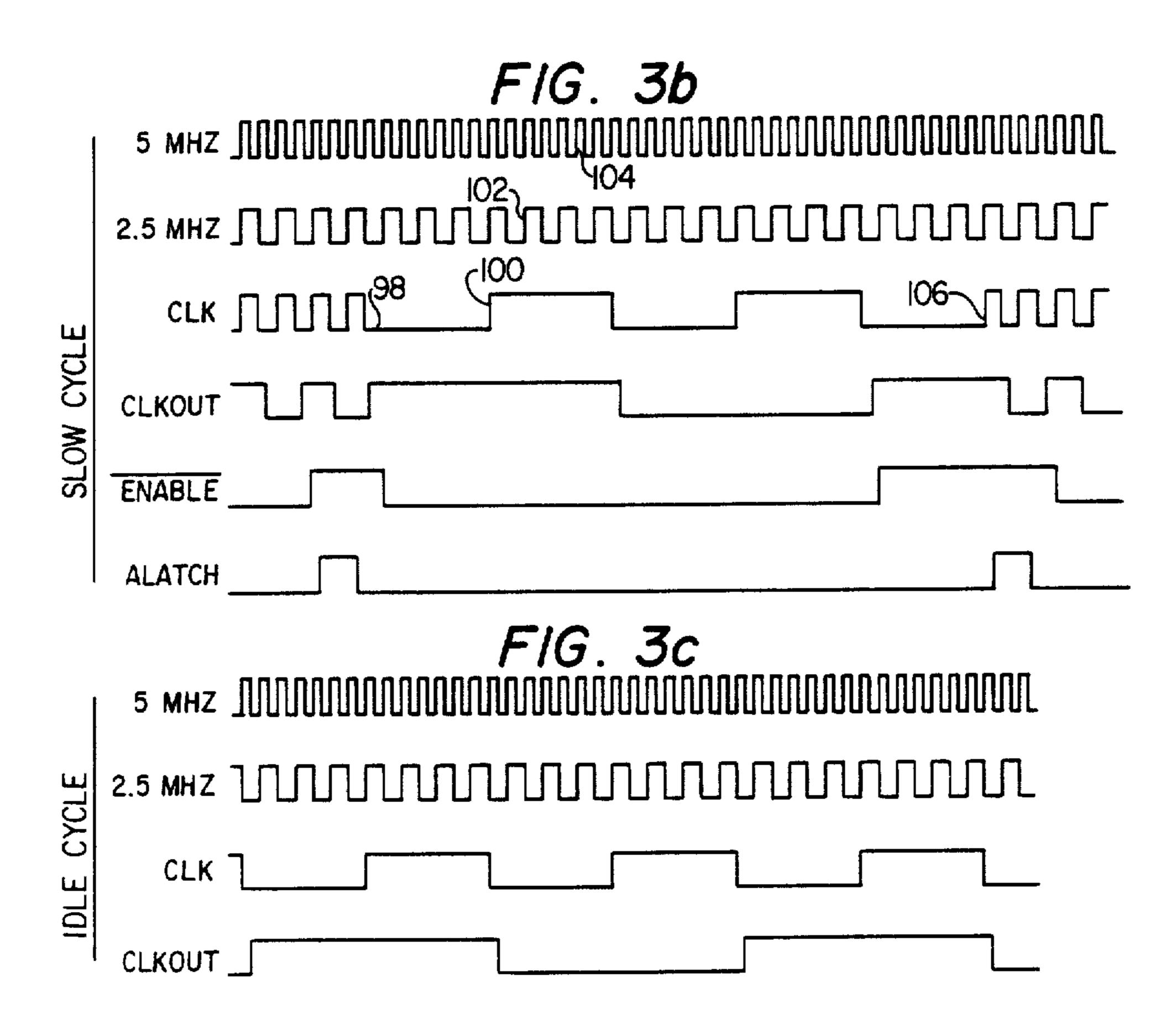
VARIABLE FREQUENCY MICROPROCESSOR CLOCK GENERATOR
