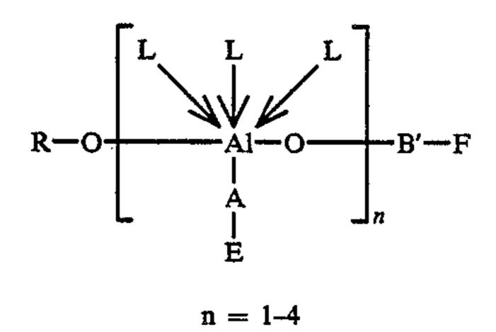
Wherein n=1-4; RO is alkoxy or aryloxy containing 1-6 carbon atoms; L are ligands and their number is 60 equal to 1, 2, or 3; A—E and B¹—F are longer chain radicals containing 12-20 or more carbon atoms, with ring and/or branch chain steric hindrance able to wrap with the chains of polymer molecules, or containing functional groups which can react with polymer molecules.
