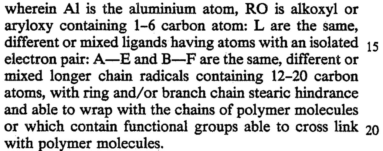
2. The aluminate coupling agent as in claim 1, Wherein the number of radicals connected with aluminum atom is 4-6.
