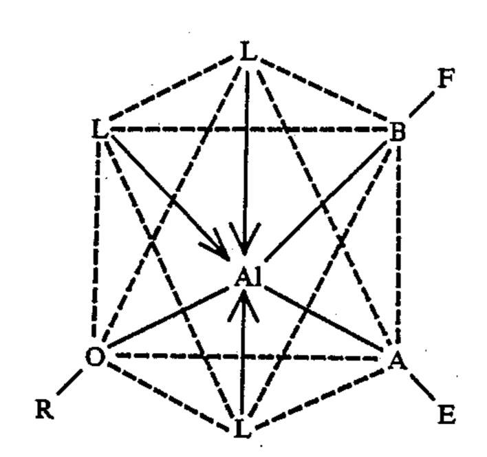
wherein Al is the aluminum atom, RO is alkoxy or aryloxy containing 1-6 carbon atoms, L are the same different or mixed ligands having atoms with an isolated election pair: A-E and B-F are the same, different or mixed longer chain radials containing 12-22 carbon atoms, with ring and/or branch chain steriric hindrance and able to wrap with the chains of polymer molecules or which contain functional groups able to cross link with polymer molecules.
