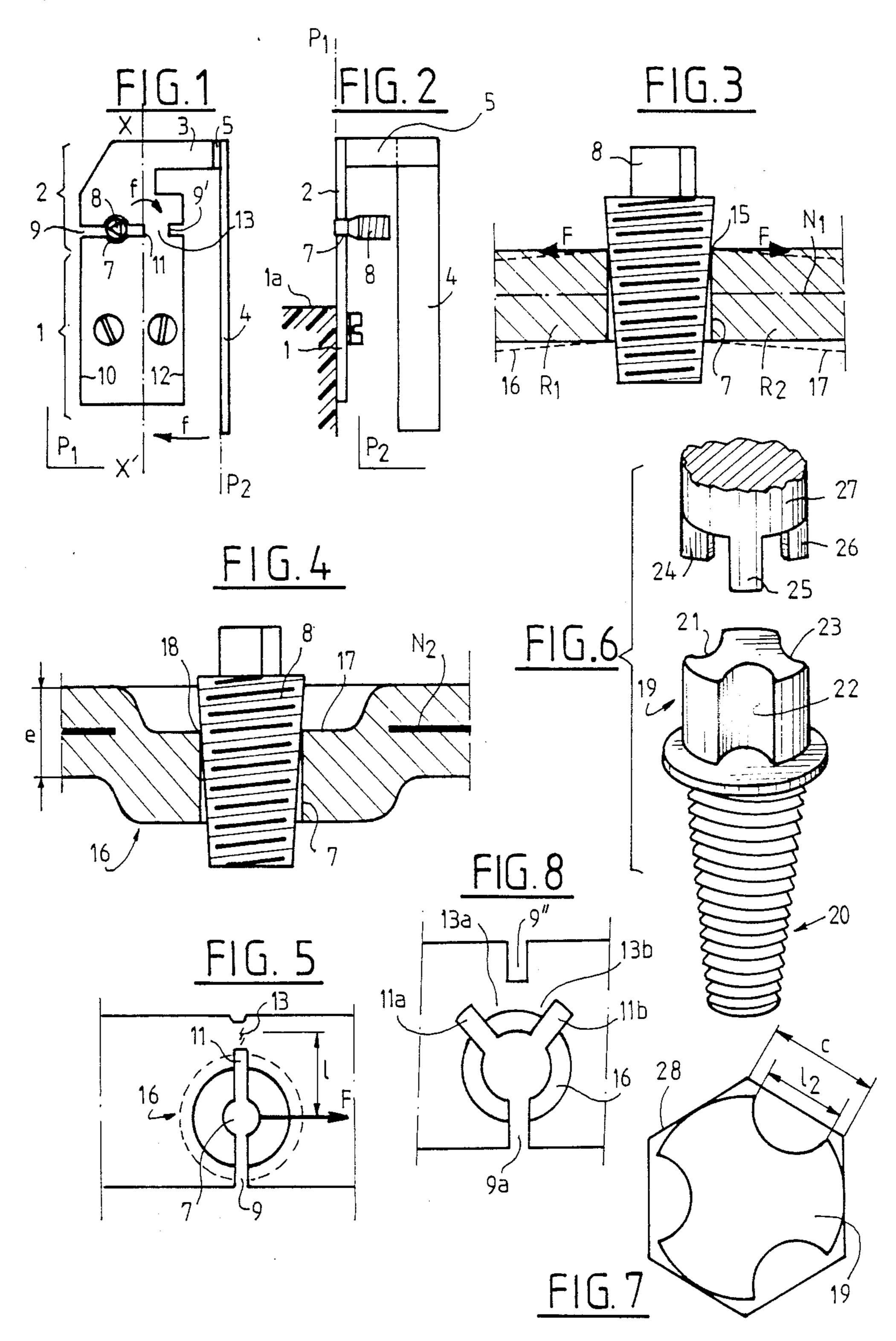
DEVICE FOR ADJUSTING THE RELATIVE POSITION OF TWO PARTS OF THE SAME PIECE BY DEFORMATION, BY MEANS OF A CONICAL SCREW, OF AN INTERMEDIATE ZONE CONNECTING THESE TWO PARTS TOGETHER
