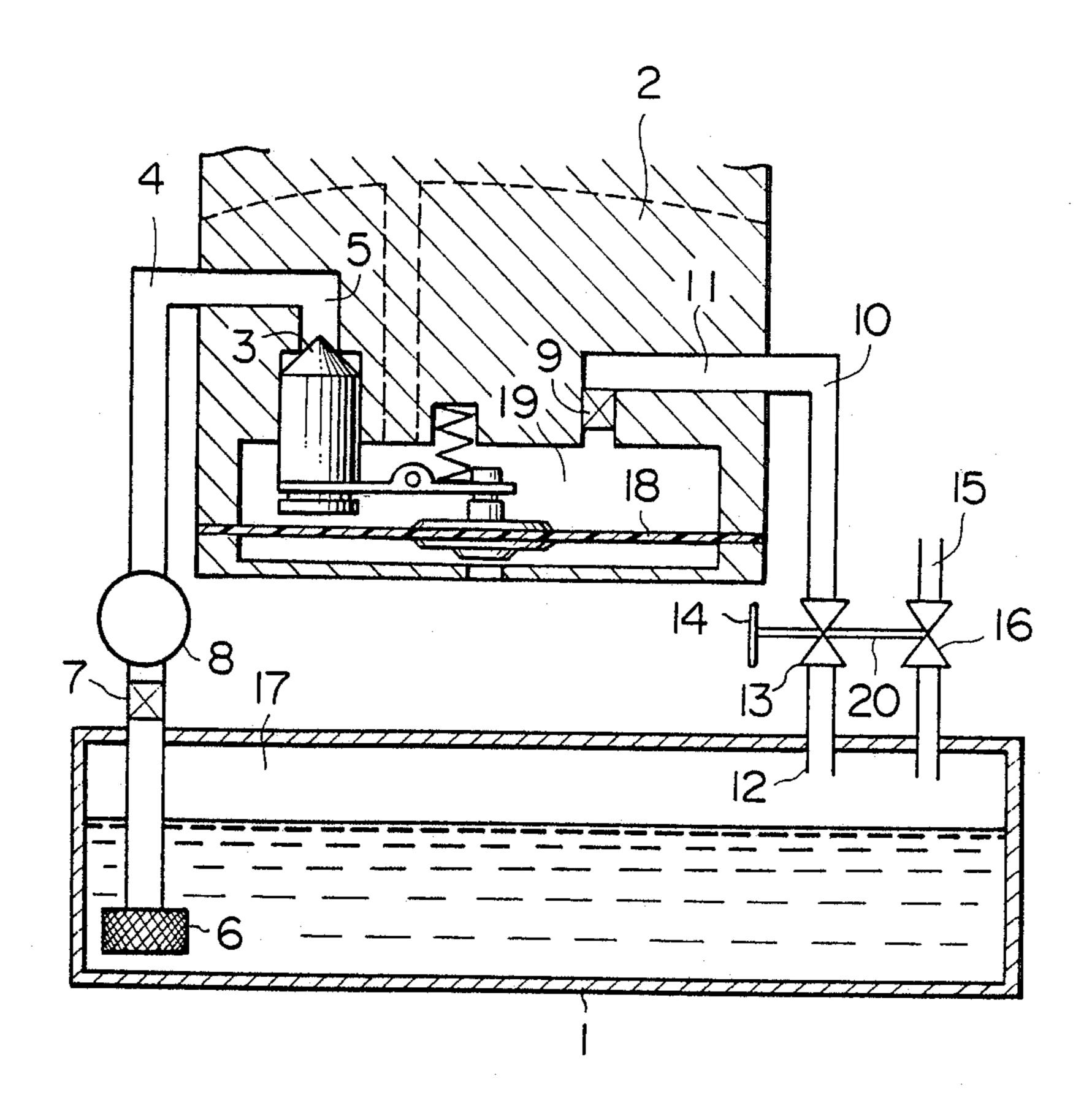
nected to a release valve so that the communication valve and the release valve are opened and closed si-
