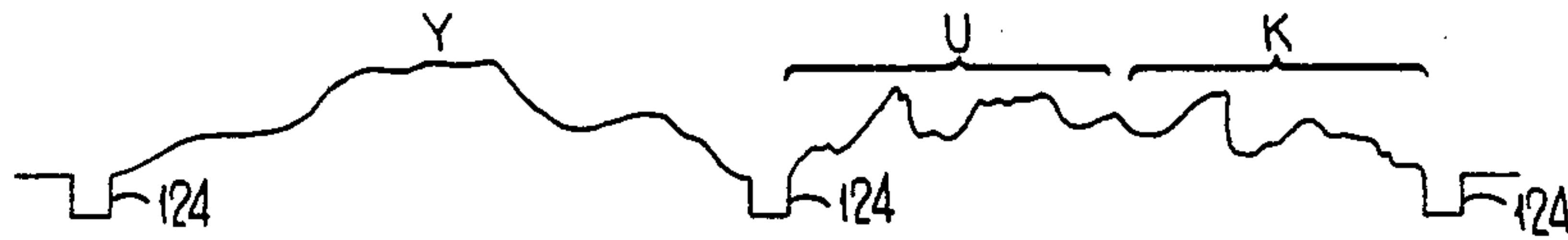
FIG 12B MULTIPLEXED ANALOG COMPONENTS
