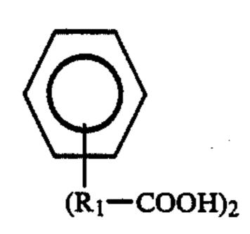
where  $R_1$  is an alkyl group having from 0 to about 5 carbon atoms and include diacids such as terephthalic and isophthalic acid.
