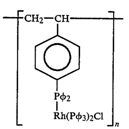
wherein  $\phi$  represents a phenyl group and wherein n represents an integer. The polymeric catalyst can be utilized in a fixed bed for hydrogenation on a continuous basis or distributed throughout a mixture of the polymer being hydrogenated in the case of a batch process. The hydrogenation process of this invention must, of course, be conducted in the presence of hydrogen gas.
