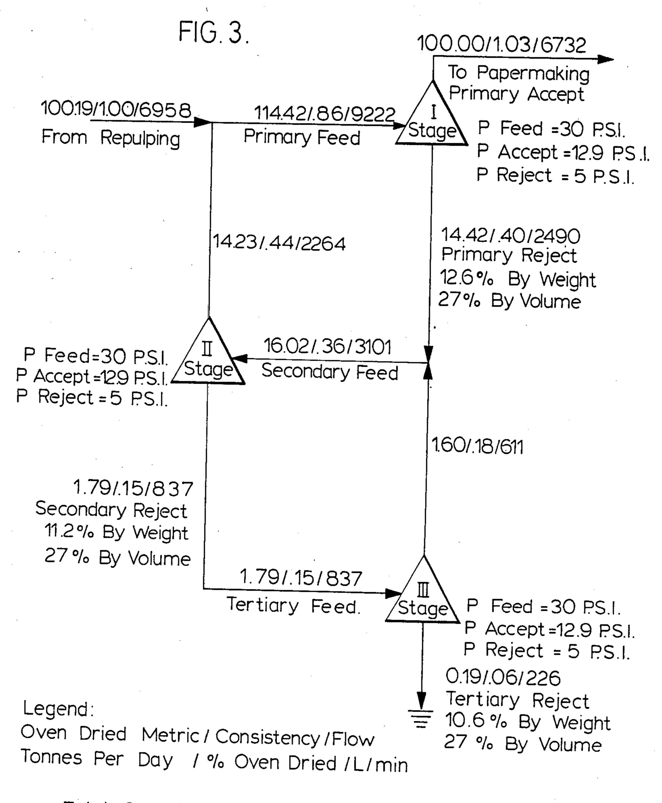
Total Capacity Required: 9222+3101+837=13,160 L/min.
