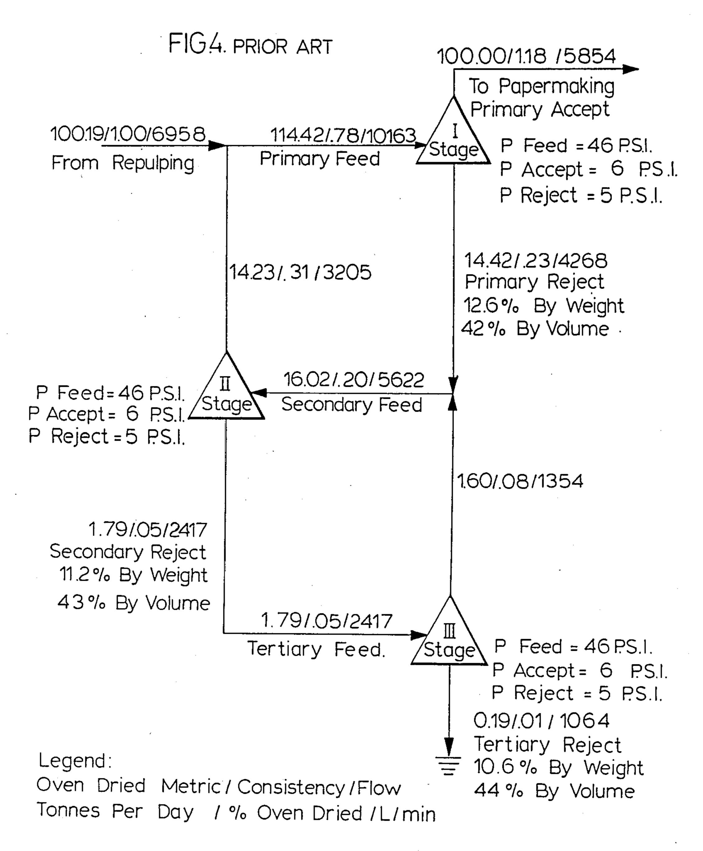
Total Capacity Required: 10163+5622+2417 = 18,202 L/min. Total Power Required:  $P = \frac{P_F \times Q}{6400} = \frac{46 \times 18,202}{6400} = 130.83 \text{ H.P.}$
