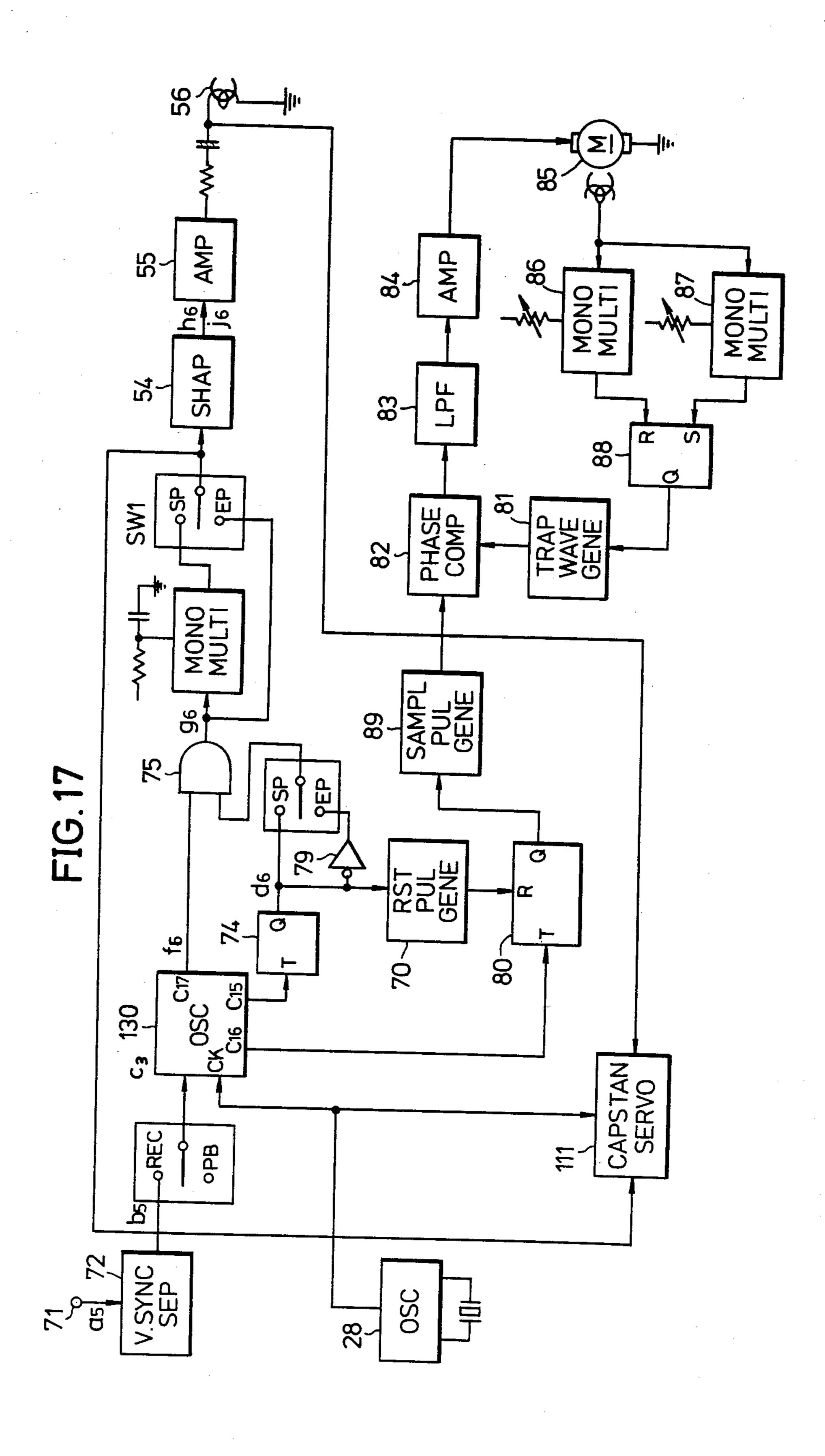
CONTROL PULSE RECORDING CIRCUIT FOR DUAL TAPE SPEED RECORDING AND REPRODUCING APPARATUSES USING TWO PAIRS OF HEADS SELECTIVELY FOR SELECTED 5 SPEED INCLUDING RECORDING DELAYED CONTROL PULSES
