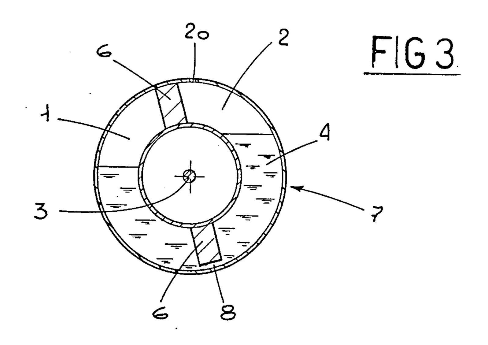
BALANCING-VESSEL TRANSDUCER WITH INTER-COMMUNICATING CHAMBERS FOR THE CONVERSION OF A PNEUMATIC SIGNAL, LOW STRENGTH NOTWITHSTANDING, INTO A QUANTIFIABLE OUTPUT OF WHATEVER NATURE
