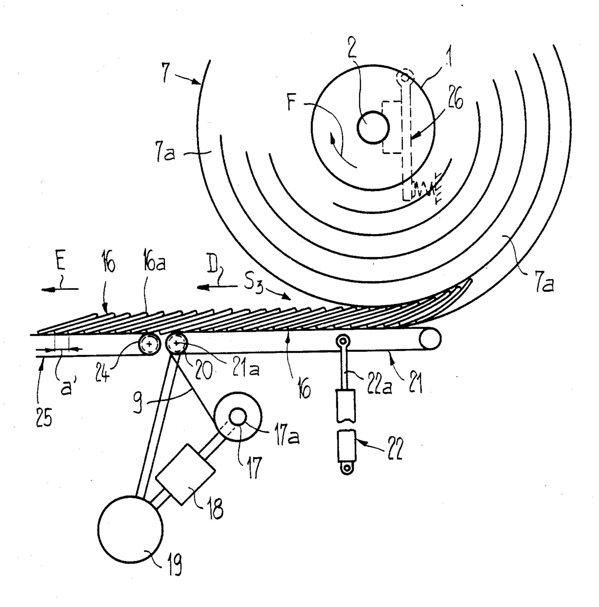
METHOD AND APPARATUS FOR FORMING MULTI-LAYER COILS FROM SUBSTANTIALLY FLAT, FLEXIBLE PRODUCTS, ESPECIALLY PRINTED PRODUCTS, ARRIVING IN IMBRICATED PRODUCT FORMATION
