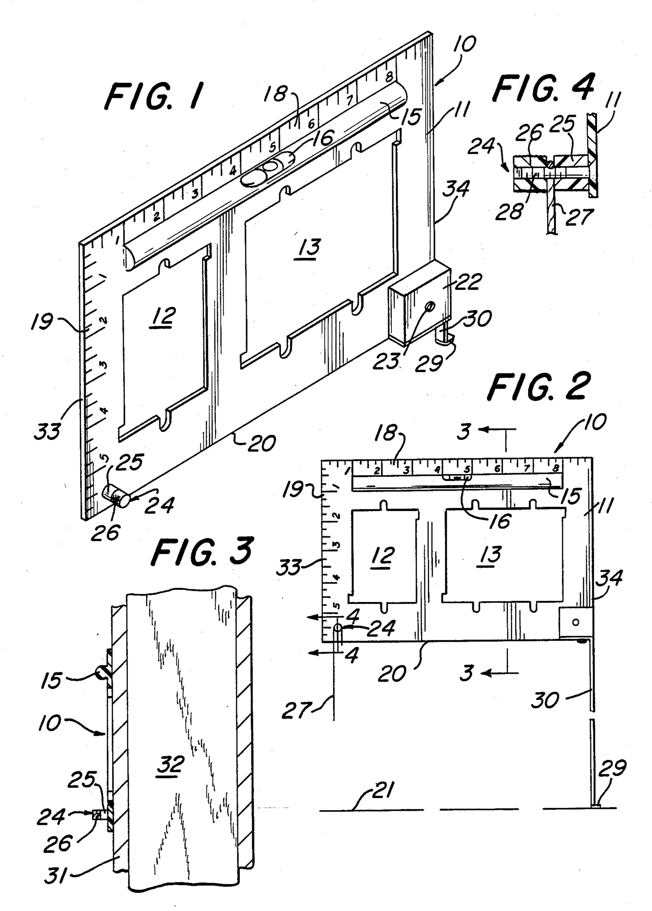
DEVICE FOR INSTALLING ELECTRIC OUTLET BOXES
