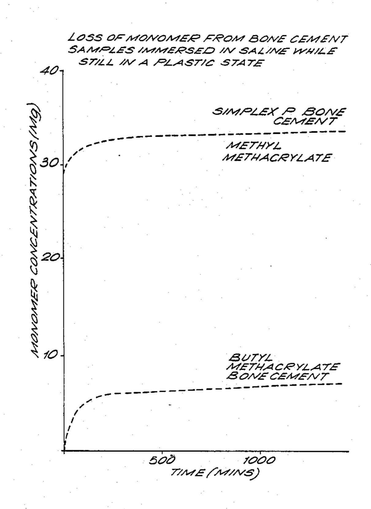
LOSS OF MONOMER FROM BONE CEMENT SAMPLES IMMERSED IN SALINE WHILE STILL IN A PLASTIC STATE
