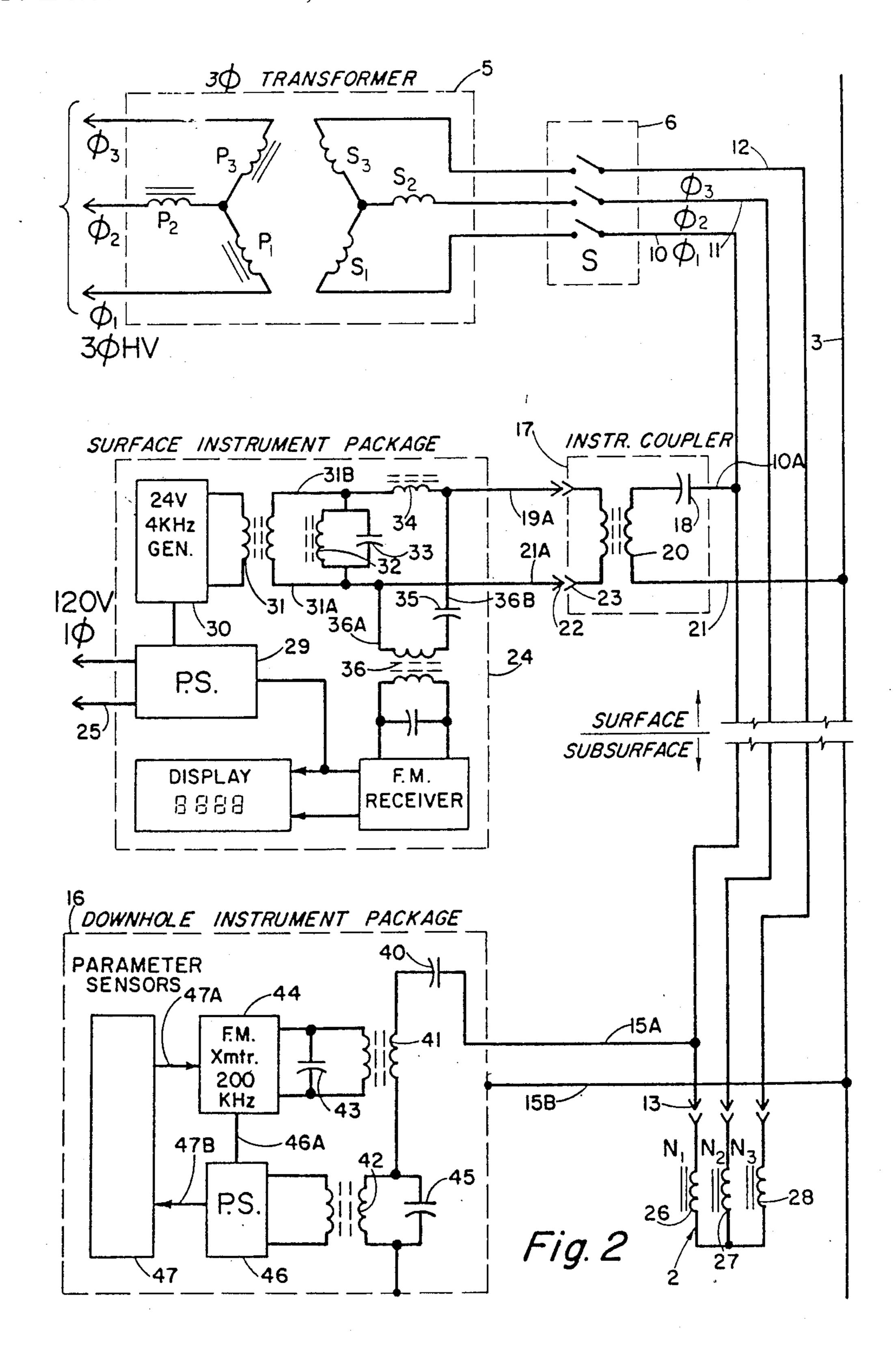
PARAMETER TELEMETERING FROM THE **BOTTOM OF A DEEP BOREHOLE**
