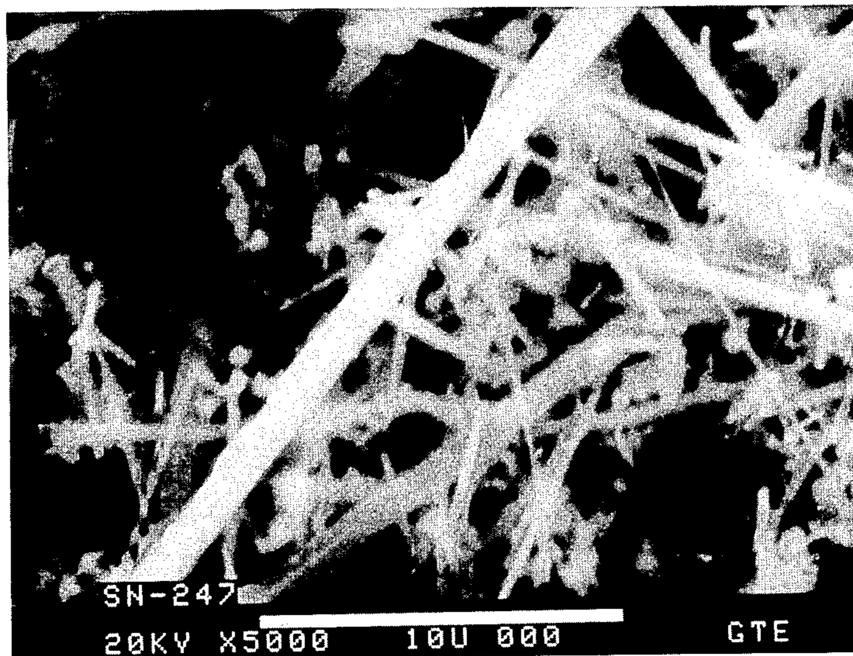
SILICON NITRIDE PRODUCED FROM AN INTERMEDIATE HAVING A BULK DENSITY OF ABOUT 0.07 g/cc
