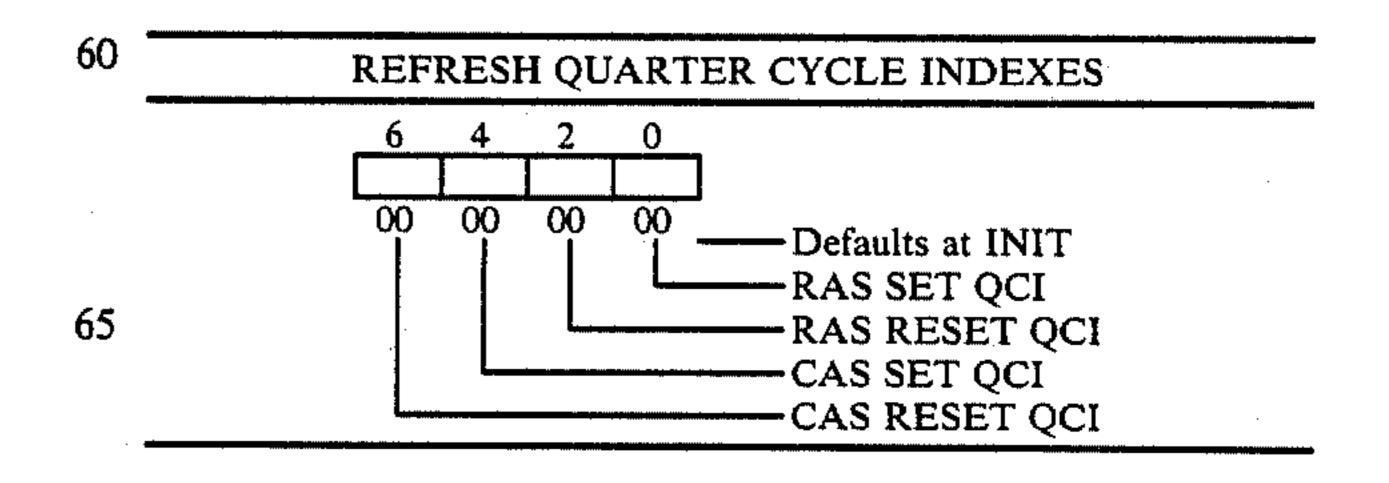
All of the fields in this register provide quarter-cycle indexes for the various Refresh access timing sequences mentioned in the diagram.
