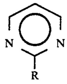
wherein R=H, CH<sub>3</sub> or C<sub>2</sub>H<sub>5</sub>, comprising the steps of (A) carrying out a gas phase reaction over a palladium-containing catalyst in the presence of a carbon monoxide-hydrogen reactant at a temperature of between 200° and 550° C., the reactant mixture comprising
