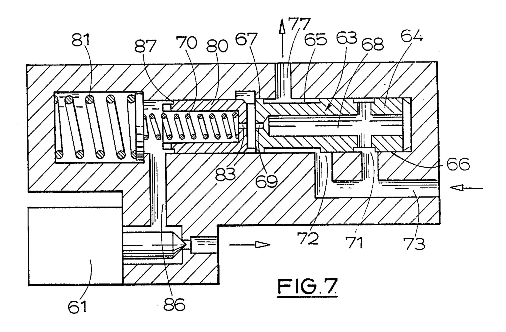
When the member comprises a piston the piston may carry a valve head for co-operation with a seating in the housing in order, partially, to close the valve assembly, and the piston hovers in such a position to define a variable orifice which reduces the release of fluid from the brake substantially at a controlled constant rate.
