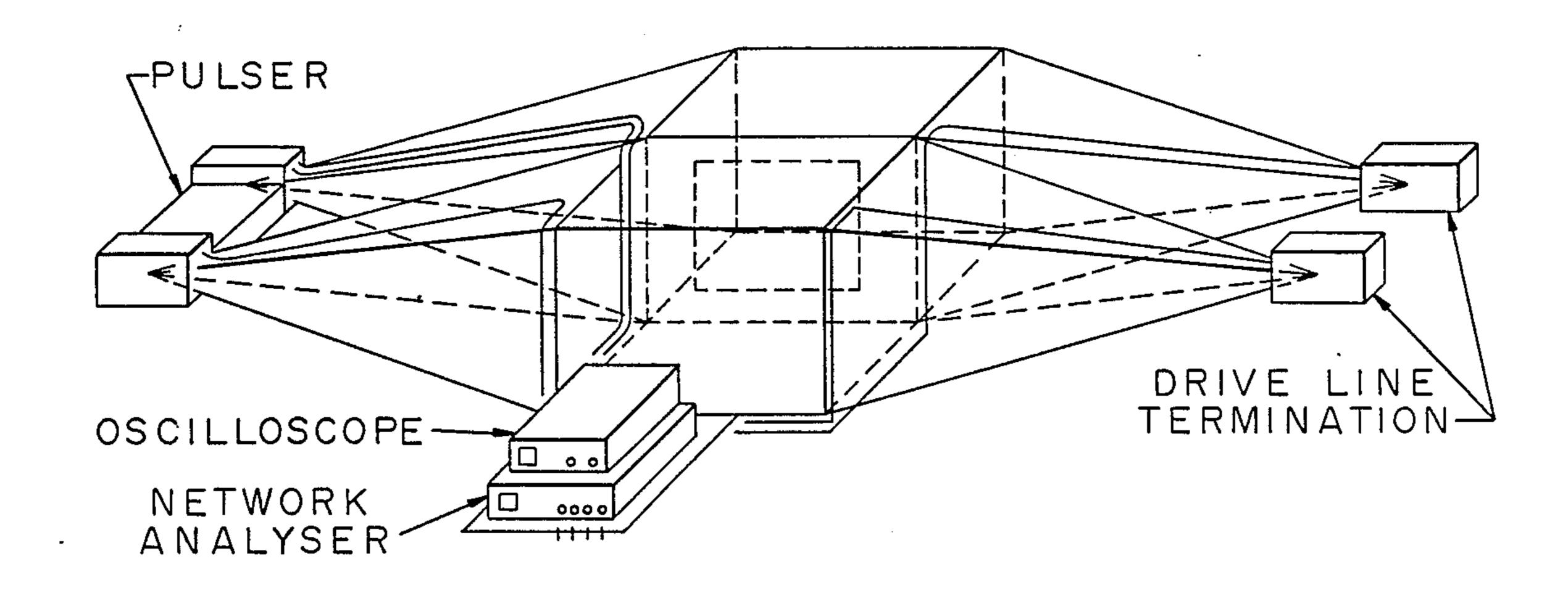
APERTURE / PENETRATION TESTER FIG. I
